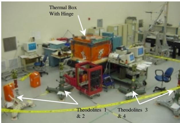
**FIGURE 3: THEODOLITE SETUP**
