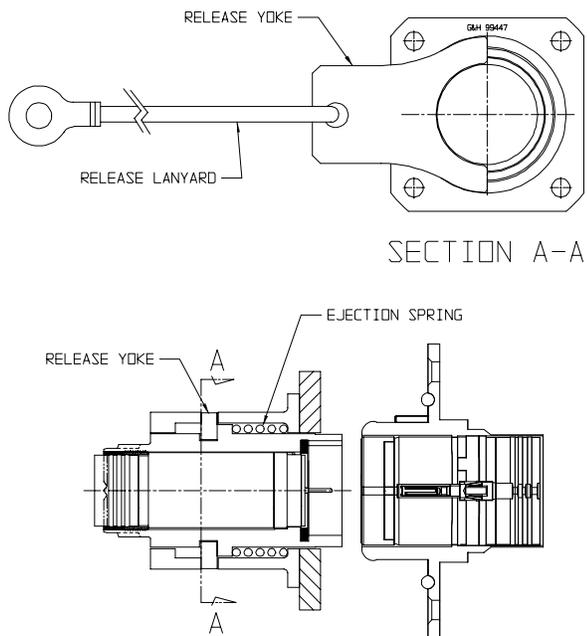
Figure 3. Initial concept of a retractable umbilical connector
