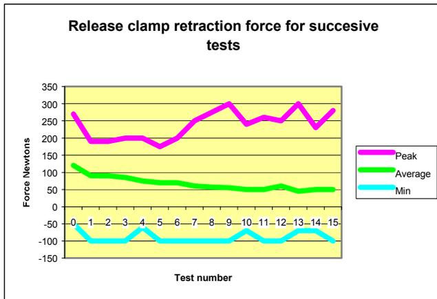
Figure 10. Release clamp retraction force during successive releases
