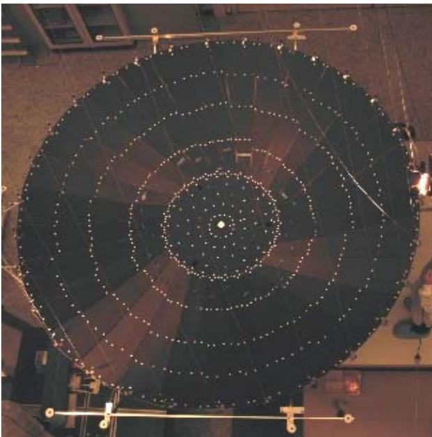
Fig. 13: Deployed Reflector during Contour Measurement.
