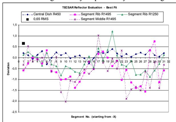
the reflector panels and for a flight model by panel screening and improvement of the panel adjustment possibility on the hinge axes so that a global rms value of about 0.3 to 0.4 mm is expected.
