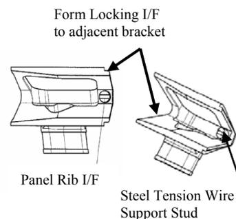
Fig. 9: Launch Locking Brackets (Top Ring Segment)
