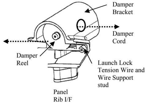
Fig. 8: Deployment Damping Device
