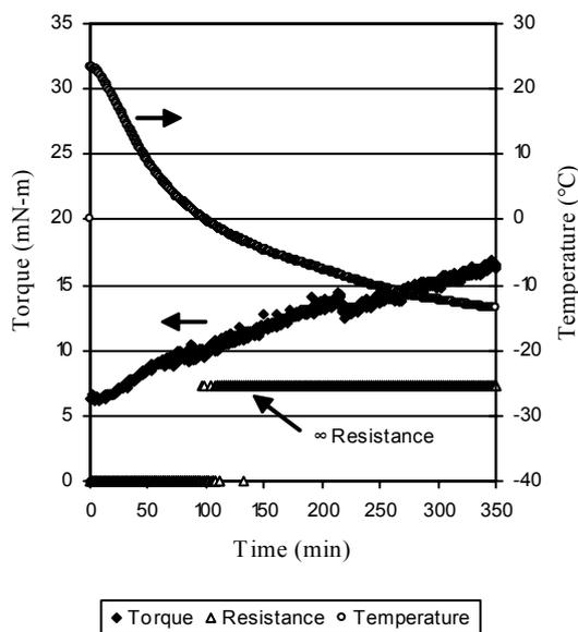
Figure 5 - Torque-temperature test for Pennzane SHF X1000
