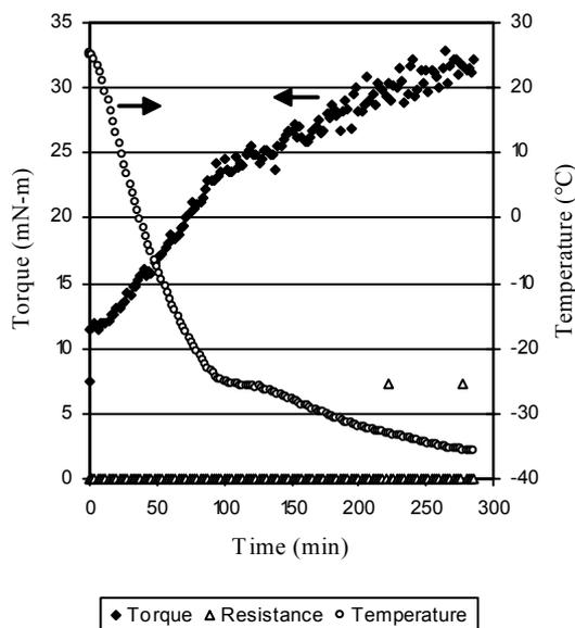
Figure 6 - Torque-temperature test for Fomblin Z-25
