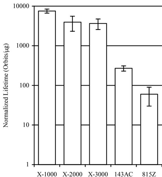
Figure 4 – Normalized lifetime for several lubricants from the spiral orbit tribometer
