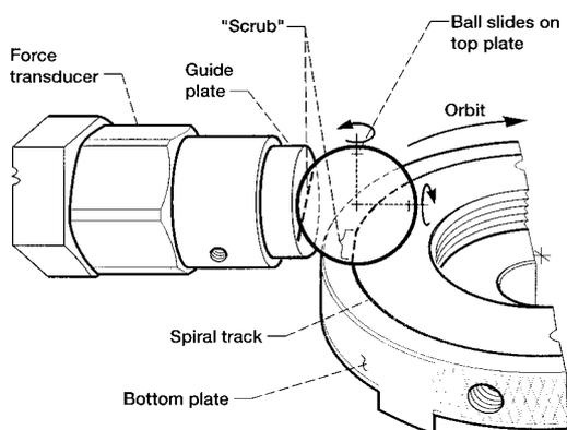
Figure 2 – Detailed view of the SOT components
