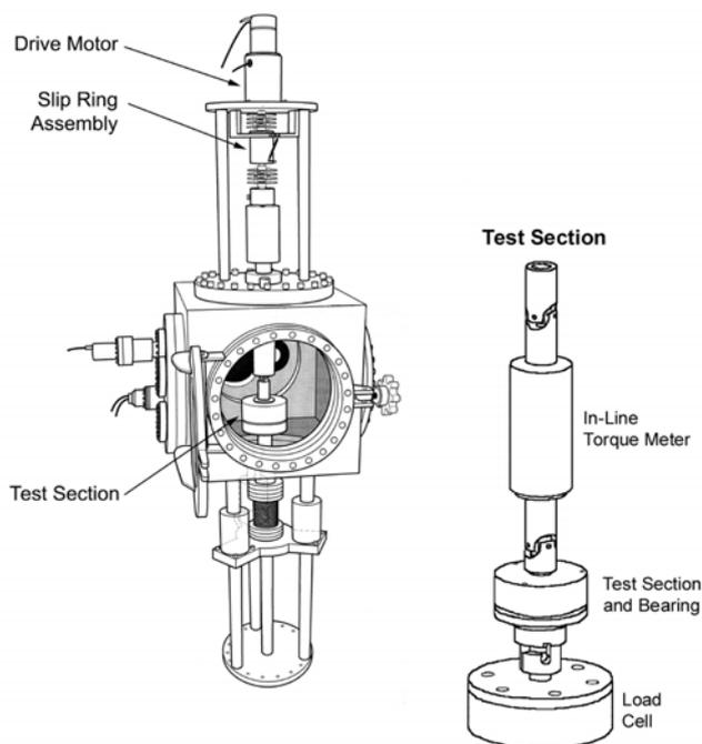
Figure 3 – Vacuum bearing rig facility and bearing fixture
