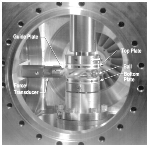
Figure 1 – Vacuum Spiral Orbit Tribometer (SOT)
