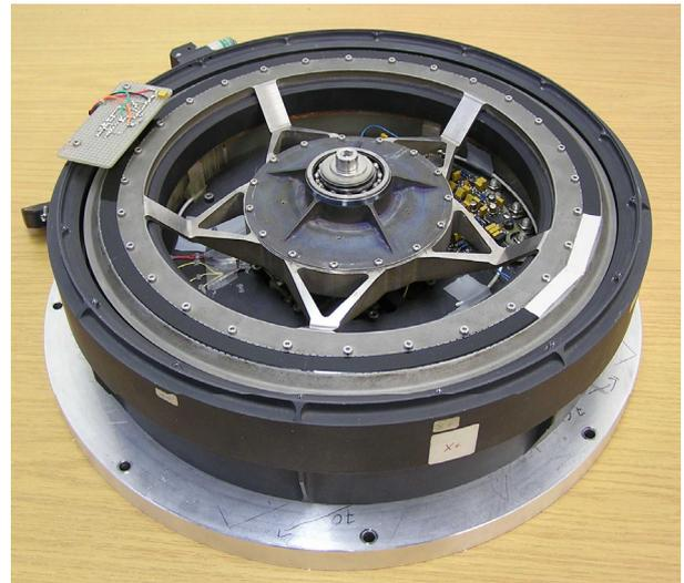
Fig. 1. Five Axes Magnetic Bearing Reaction Wheel
