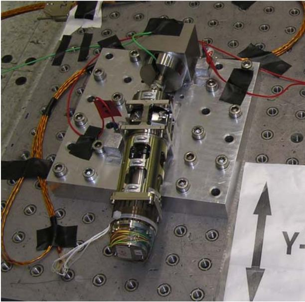
Fig. 21: Single Actuator Vibration Test Set-up with inclined orientation
