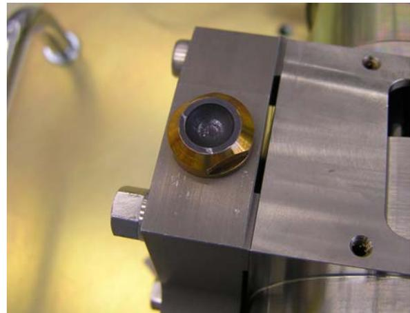
Fig. 6: PME Cup (Brass with MoS<sub>2</sub> - sprayed)
