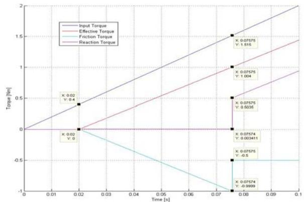
Fig. 17: Static Torque Transfer Characteristic of the Spindle.
