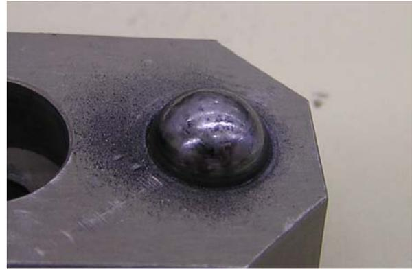
Fig 8: Ball Surface after Vibration Test
