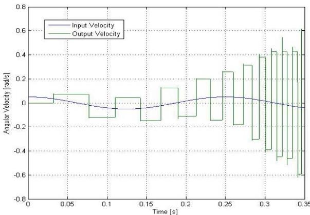
Fig. 15: Velocity Response of the gear-box with backlash
