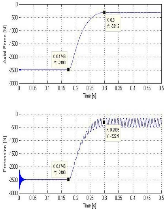
Figure 19: Axial Force and Pretension for Actuator Holding Force Simulation
