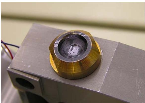
Fig. 7: Cup Surface after Vibration Test
