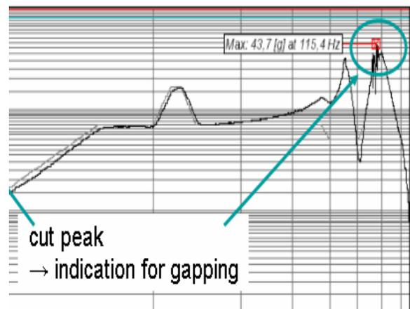
Fig. 9: Cut Peak at Sine Acceptance 2<sup>nd</sup> mode
