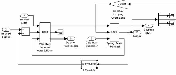
Fig. 13: Gear-Box Model
