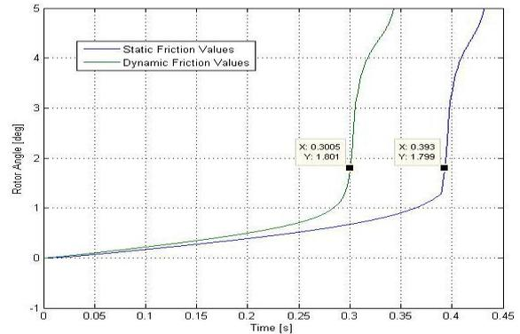
Fig. 12: Rotor Angle vs. Time for a Linearly Increasing Input Torque
