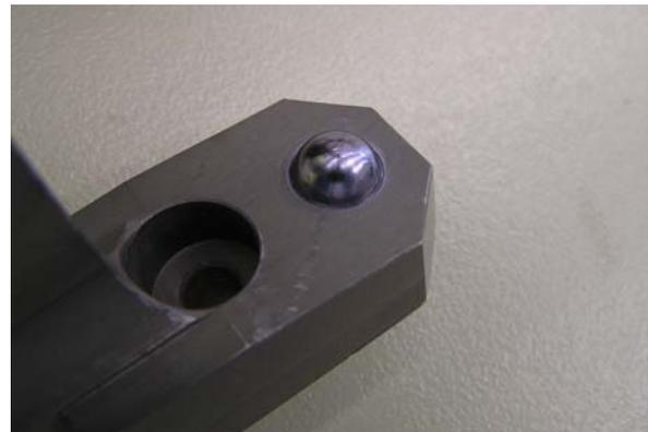
Fig. 5: PME Ball (steel with MoS<sub>2</sub> - polished)
