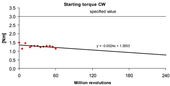
Figure 12 Life test starting torque prediction (CW shown, CCW is similar)
