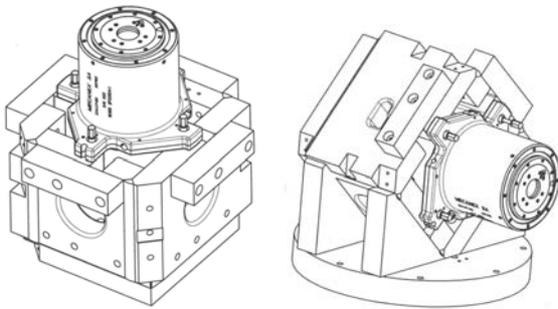
Figure 5 Vibration test fixture
