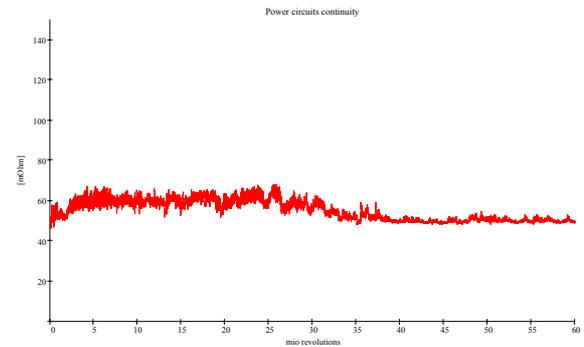
Figure 6 Life test resistance of all power circuits in series (25 ADC, 225 RPM)
