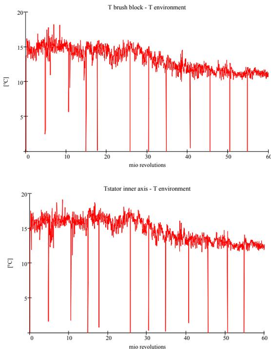
Figure 8 Life test internal temperature measured on brush block (top) and inner axis (bottom)
