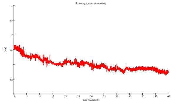
Figure 9 Life test running torque (225 RPM)
