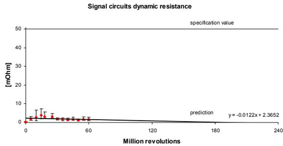
Figure 11 Life test signal circuits dynamic resistance prediction
