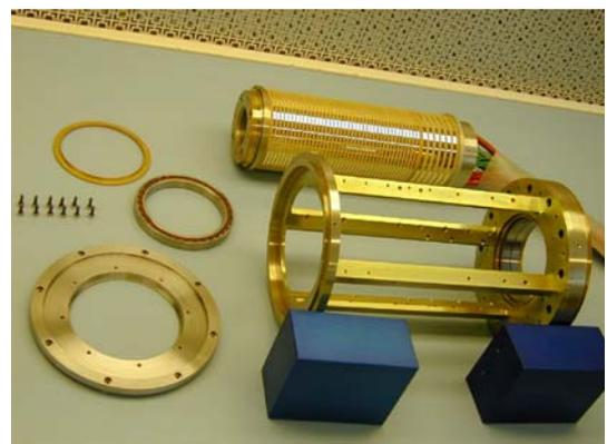
Figure 2 Rotor and stator assemblies
