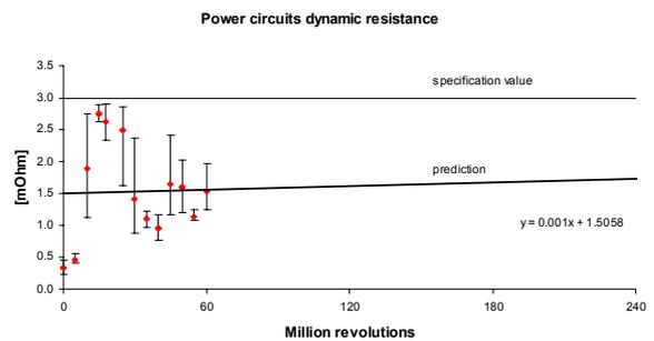
Figure 10 Life test power circuits dynamic resistance prediction
