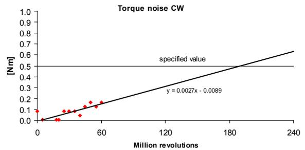
Figure 14 Life test torque variation prediction (CW shown, CCW is similar)
