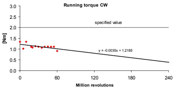
Figure 13 Life test running torque prediction (CW shown, CCW is similar)
