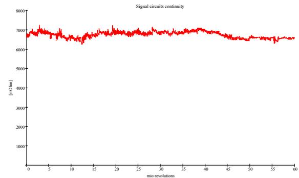
Figure 7 Life test resistance of all signal circuits in series (1 ADC, 225 RPM)
