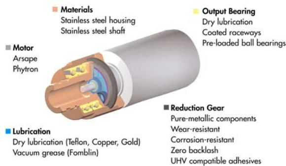
Fig. 8 Special modifications for vacuum applications
