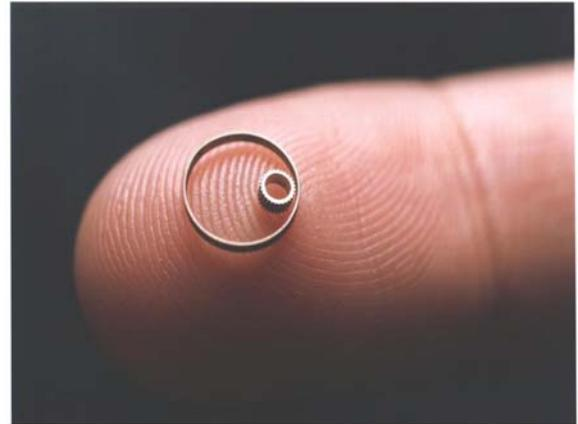
Fig. 5 Gear wheels in Nickel-Iron alloy
