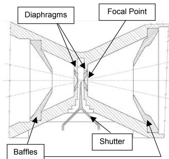
Fig. 4: LCM optical path cross-section
