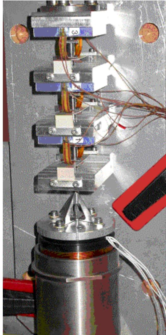
Fig. 14: LCM position sensor
