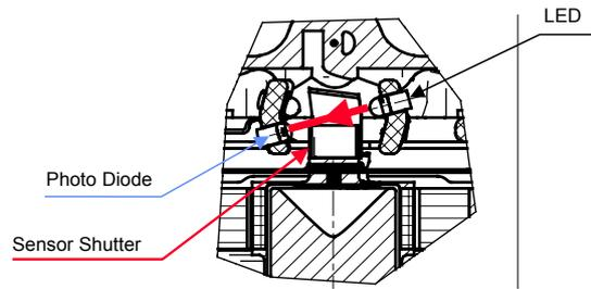
Fig. 14: LCM position sensor
