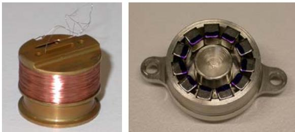
Fig. 10a: Parts of the custom made LCM voice coil actuator (Breadboard version)
