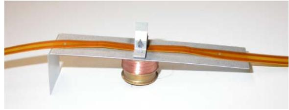
Fig. 10b: Parts of the custom made LCM voice coil actuator (Breadboard version)
