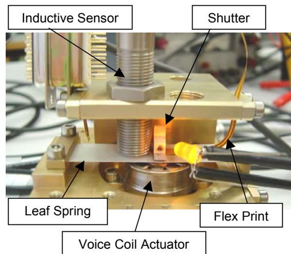
Fig. 11: Breadboard Test Setup
