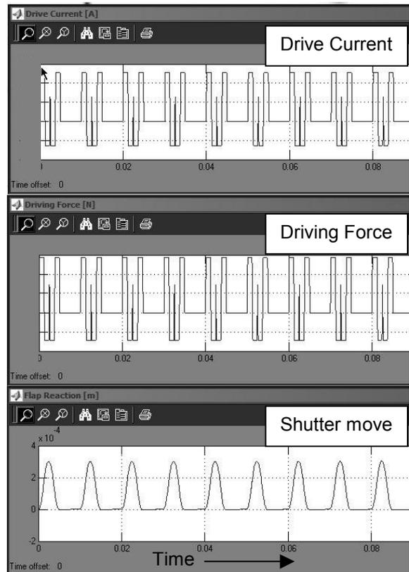
Fig. 9: Current Waveform and Shutter Movement
