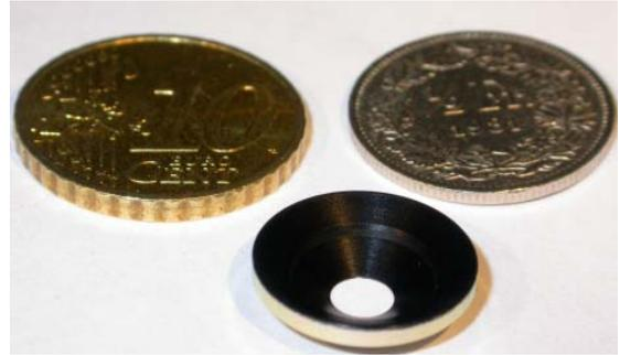
Fig. 8: LCM large straylight baffle
