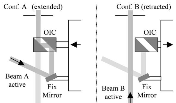
Fig. 1: FFM Configurations
