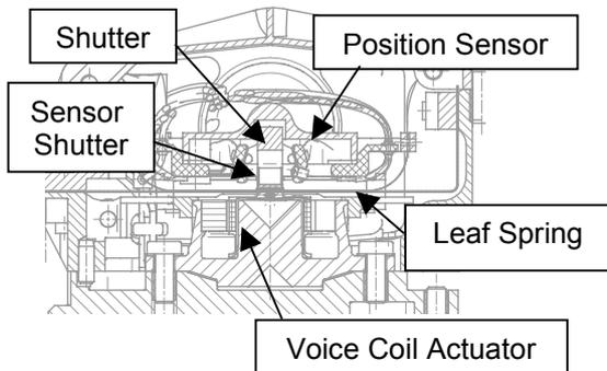
Fig. 6: LCM cross-section B
