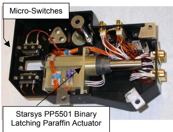
Fig. 3: FFM Hardware (Bottom View)
