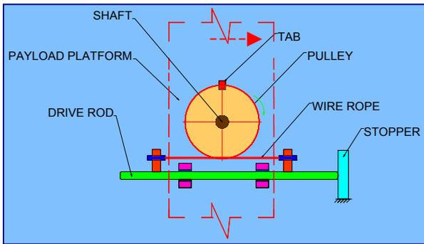
Fig. 5 Declination Drive Principle
