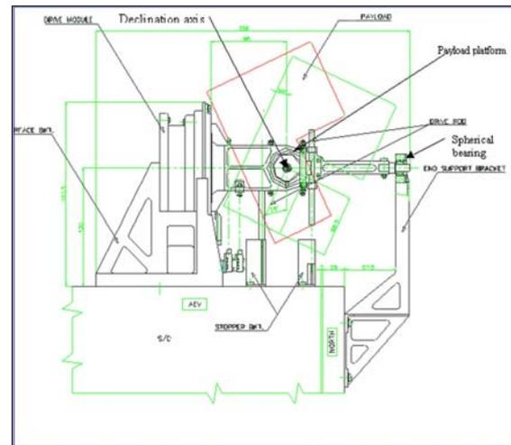
Fig-3 Sun Tracking Mechanism
