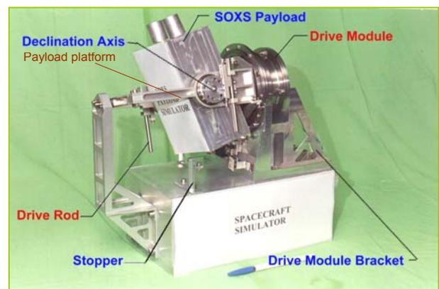
Fig.4 Sun tracking Mechanism assembly
