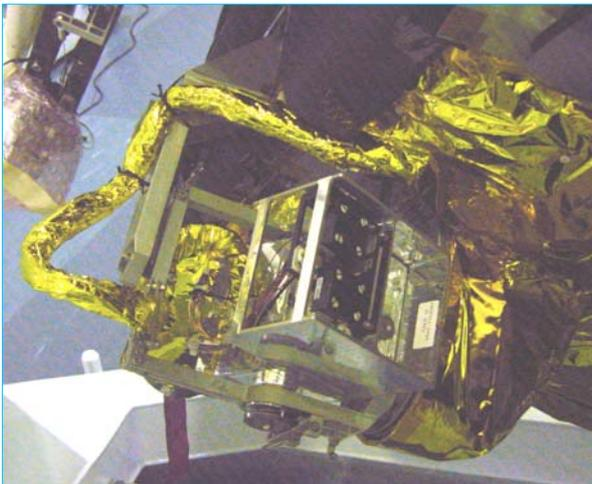
Fig. 9 Mechanism on Spacecraft with Payload Package and harness loop
