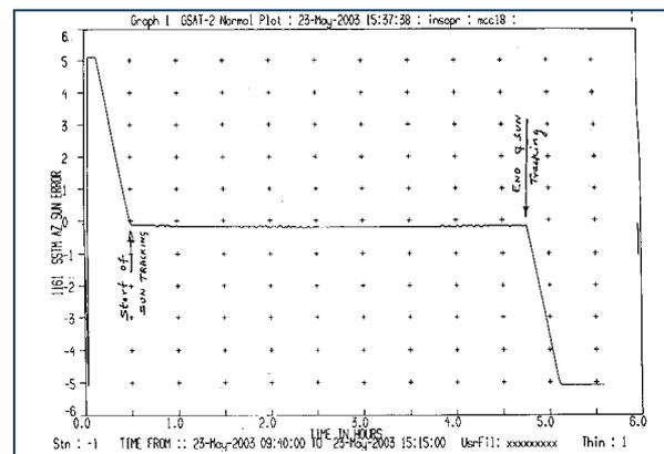
Fig. 10 Sun Sensor Angle during tracking
