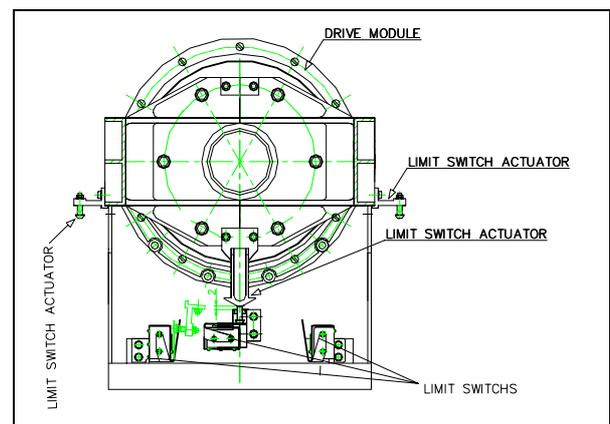
Fig. 8. Limit-Switches Mounting Detail
