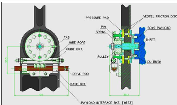
Fig. 6 Friction hold on declination trunion
