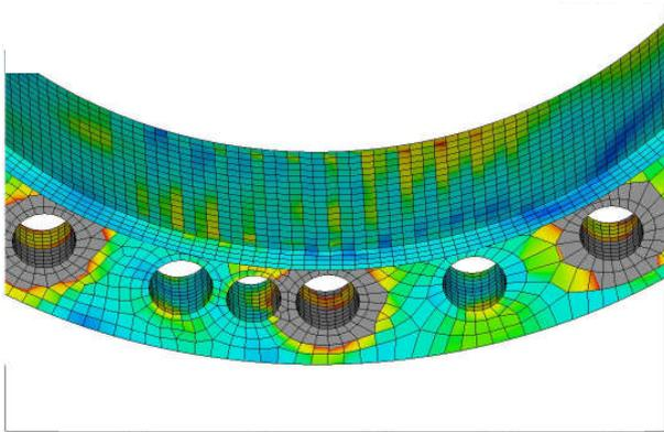
Figure 3: FE-calculation of the Circular Spline
