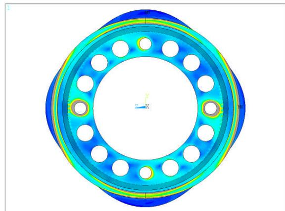
Figure 2 FE-calculation of the Wave Generator
