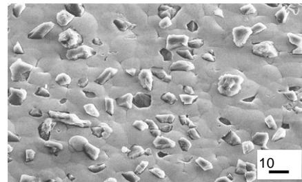
Figure 10: Surface structure of friction shim.
