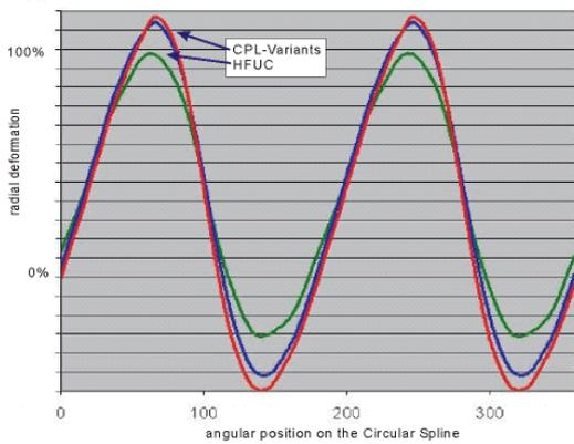
Figure 4: Relative radial deformation on the Aluminum CS over circumference
