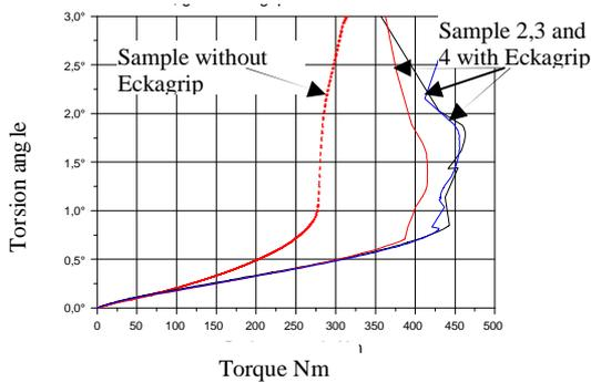
Figure 12: Comparison of the output torsion stiffness of HFUC with and without friction shim.
