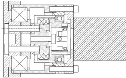
Figure 13: Gear in gear concept
