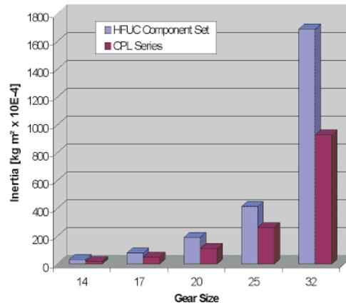
Figure 6: Inertia comparison for CPL vs. HFUC
