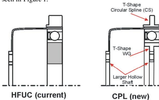
Figure 1: Identified changes for weight reduction
