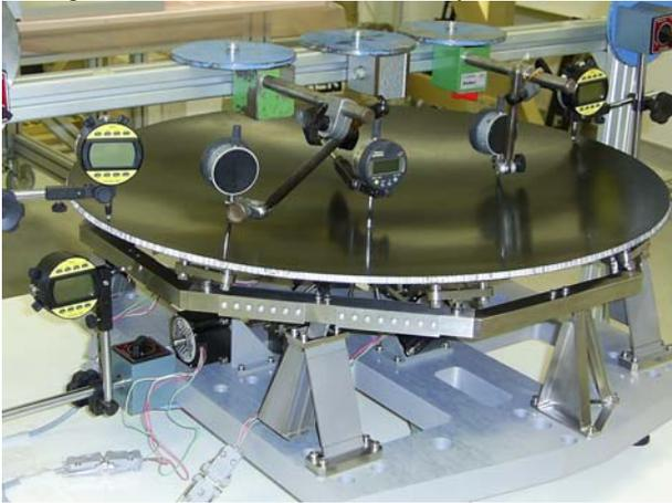
Figure 14. Dial gauges configuration for initial tests
