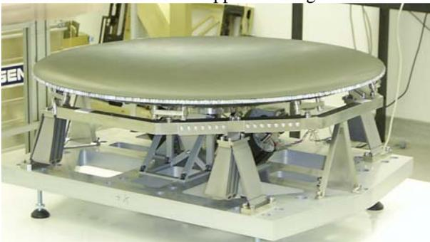
Figure 3. SubReflector Assembly configuration
