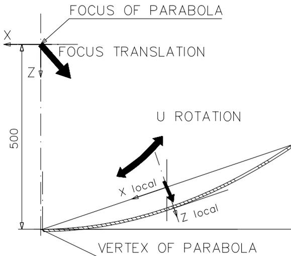
Figure 2. Subreflector reference Axis
