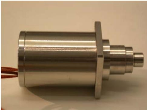
Figure 13: Rotational micro positioning system based on a UHV suitable Micro Harmonic Drive<sup>®</sup> gear box (Source: DESY, Hamburg)
