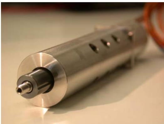
Figure 14: Linear micro positioning system (Source: DESY, Hamburg)
