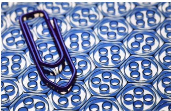
Figure 2: Micro gear wheels fabrication on a silicon wafer
