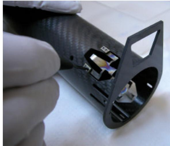
Figure 6.1 Fitting of Latches to Tube
