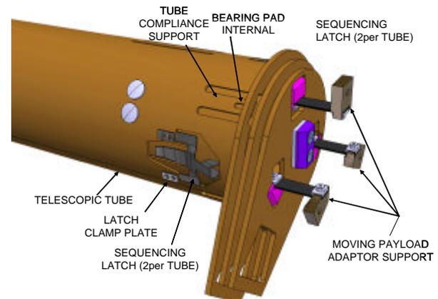
Figure 4.2: Tube outboard end showing cantilever springs supporting contact pads
