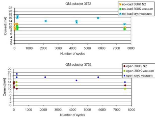
*Figure 6: Measured actuator starting current for different conditions (warm vs. cold, no load vs. cover load, nitrogen atmosphere vs. vacuum).*
