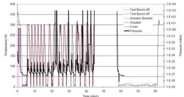
*Figure 10: Evolution of pressure and temperature during the QM thermal vacuum tests.*
