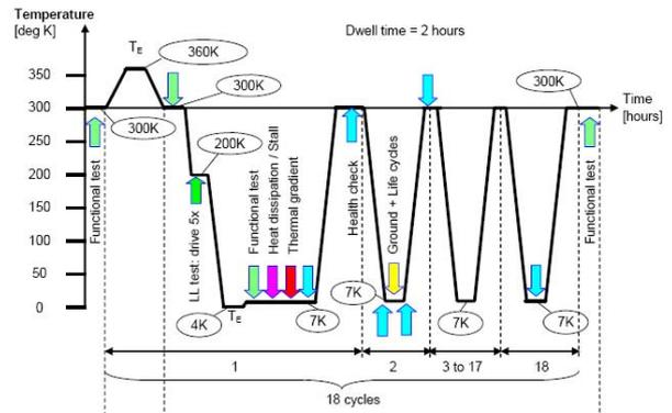
*Figure 8: Thermal cycle sequence with the CCC Qualification Model.*
