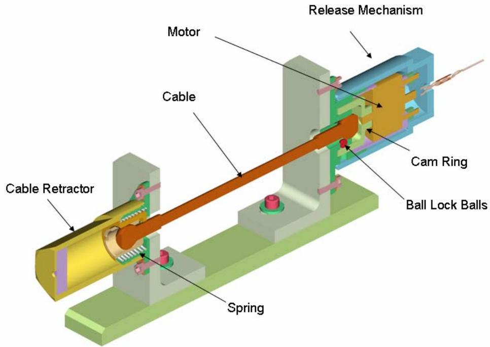
Figure 10. Electrically Powered Cable Release Cross Section
