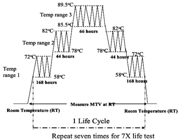
Figure 11– Temp. Profile Based on Mission Prediction
