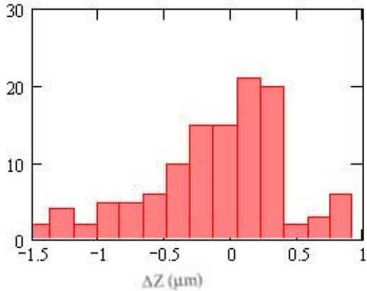
**Figure 15: Histogram of final axial position dispersion of the TM (sample: 119 grabbing's)**
