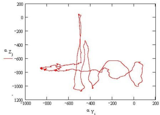
Figure 14: Rotational movement of the TM during grabbing approach ( $\alpha_Z$  and  $\alpha_Y$  are rotations in  $\mu$ rad around Z and Y respectively).
