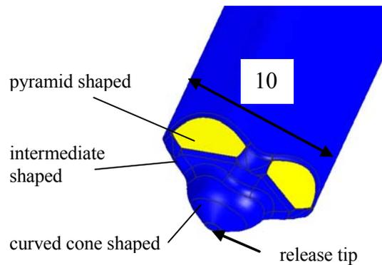
**Figure 5: Grabbing finger with pyramidal shape**
