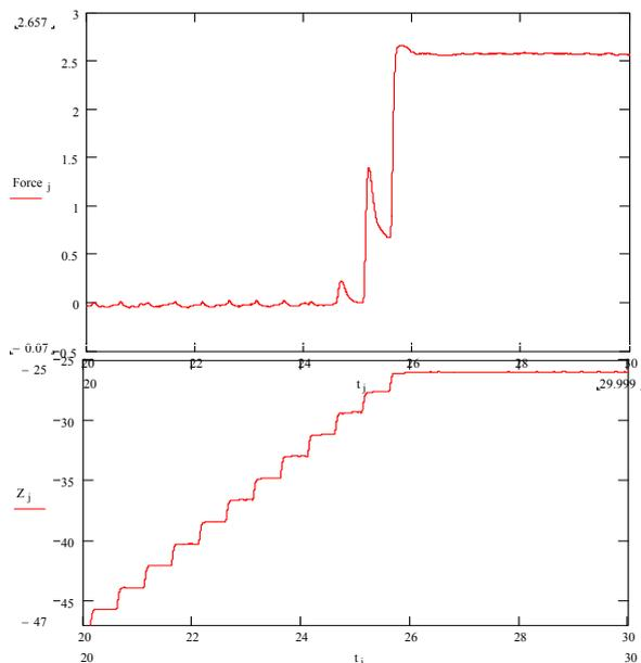
Figure 12: Grabbing finger axial force and displacement at grabbing position
