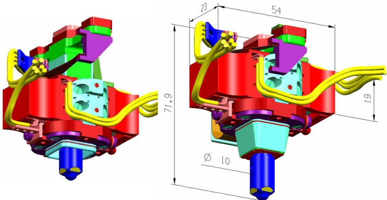
Figure 2: General GPRM design in retracted and extended grabbing finger position
