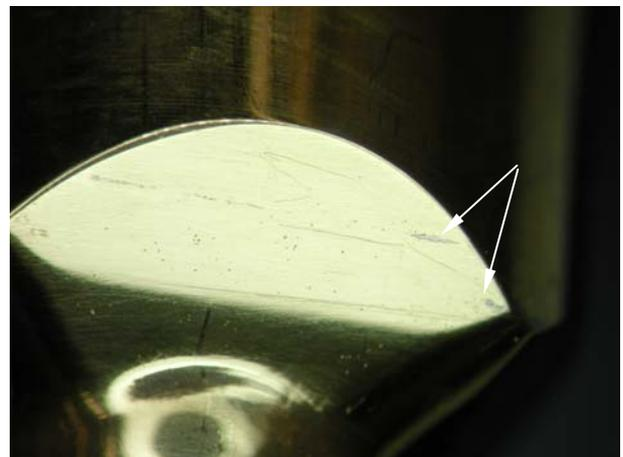
**Figure 19: Grabbing finger pyramid after life test, small damaged areas marked**
