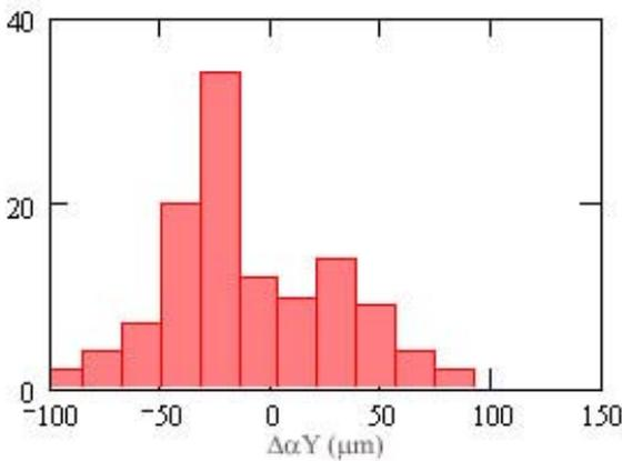
**Figure 16: Histogram of final angular position dispersion about Y of the TM (sample: 119 grabbing's)**
