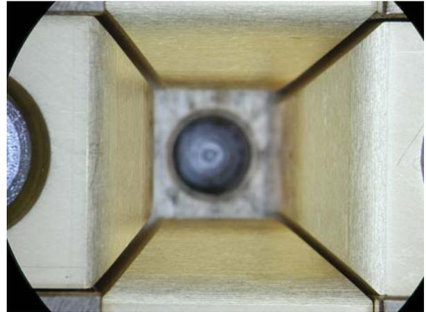
**Figure 18: Dummy recess after life test. Gold plating not damaged**
