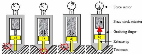
**Figure 7: Hand over and release sequence**
