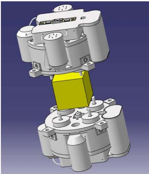
Figure 1: Parts of the Caging mechanism
