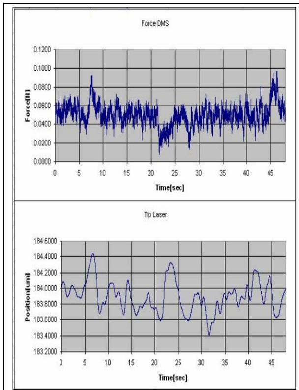
**Figure 9: Force and Position read-out during hand-over testing**
