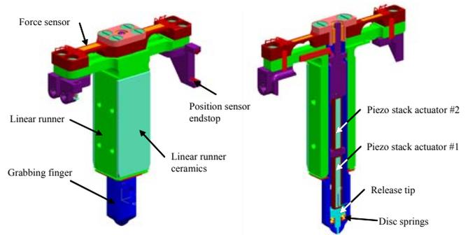
**Figure 4: Grabbing finger unit with force sensor and release tip**
