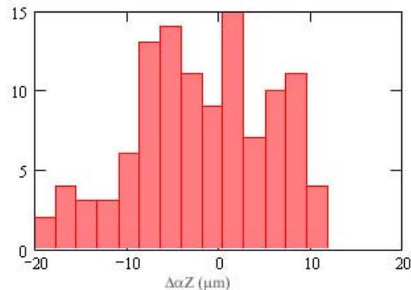
**Figure 17: Histogram of final angular position dispersion about Z of the TM (sample: 119 grabbing's)**
