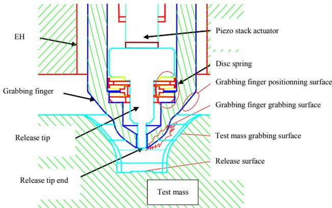
**Figure 6: Grabbing finger with release tip**
