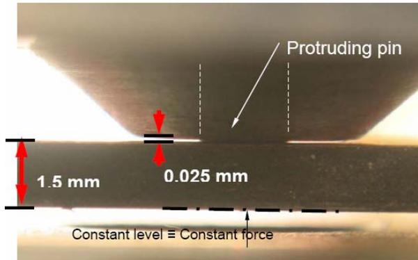
**Figure 8: After hand-over - release pin extended**
