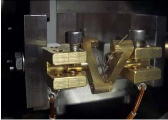
Figure 5: Mounted crossed wires ready for test
