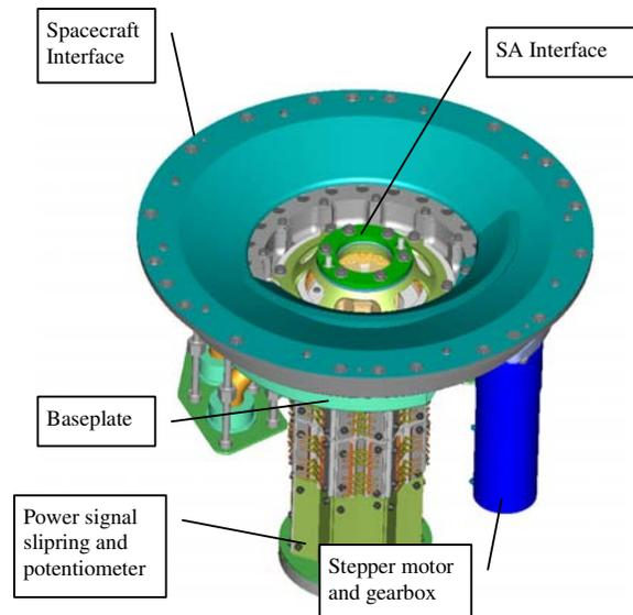
Figure 1, High Power Solar Array Drive mechanism
