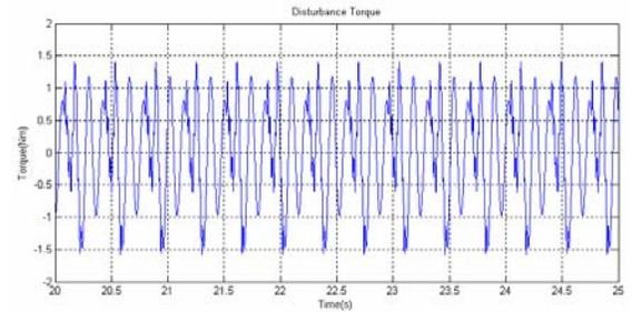
Figure 14, 20 RPD Simulated Disturbance Torque
