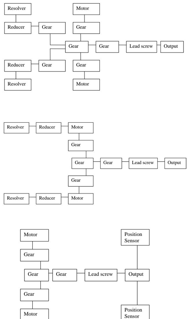
Figure 2 Components arrangement options
