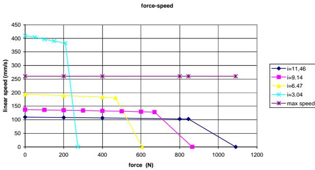
Figure 9 different gear ratios comparison
