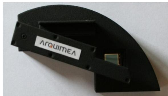
Figure 1. Top view of the SMA Rotary Actuator.
