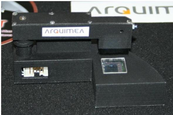
Figure 5: Front view of the SMA Rotary Actuator.
