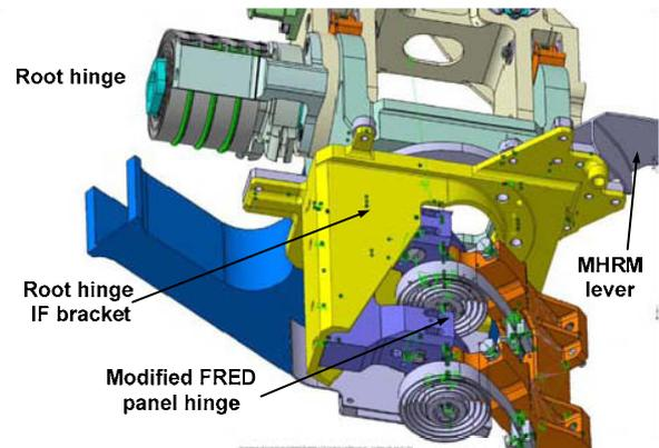
Figure 7. Interface to the Solar Array and MHRM
