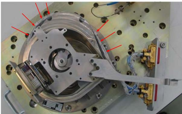
Figure 10. Cable harness of the QM
