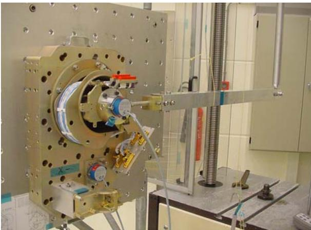
Figure 13. Stiffness test (X-axis) with inclinometers
