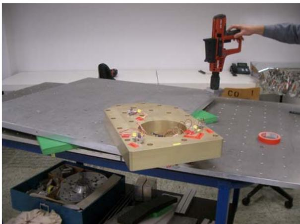
Figure 18. Shock test preparation with dummy
