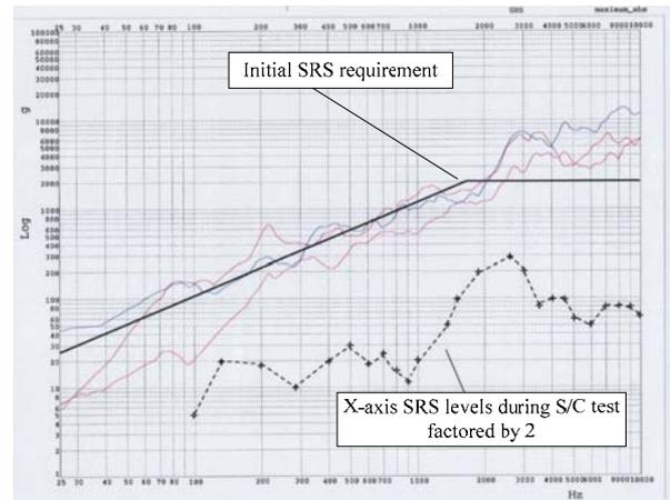
Figure 19. X-axis shock test results
