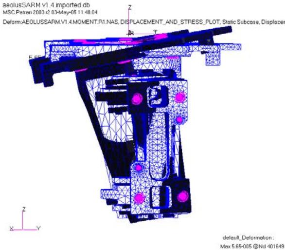
Figure 5. Root hinge IF bracket and hinge FEM
