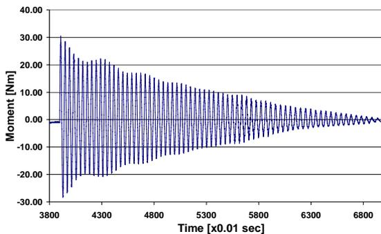
Figure 15. QM SARM deployment shocks
