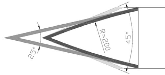
Figure 7 Geometry of three different penetrators tips; the one with 45° conical angle (bright line), the one with 25° conical angle (mid gray line) and the one which curved conical envelope (circular section with 200 mm radius) (dark line).
