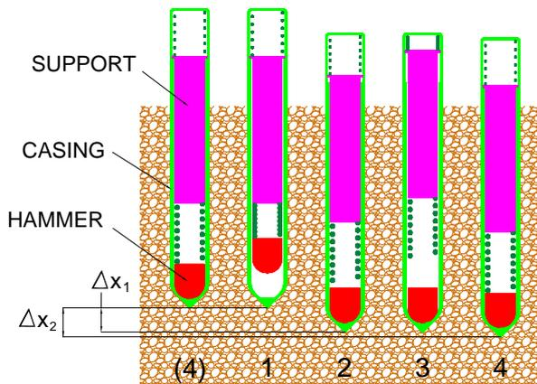
Figure 1 Schematic principle of operation of the mole
