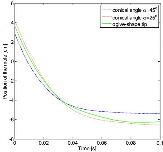
Figure 9 The penetration progress obtained for the tips presented in Fig. 7. The dashed blue line corresponds to the 45° conical angle penetrator, the dotted red line to the 25° conical angle penetrator and solid line corresponds to the ogive-shaped tip.
