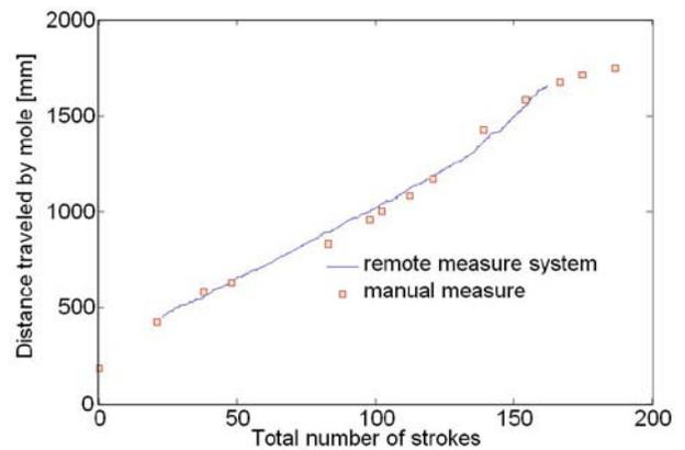
Figure 11 Dependence of insertion progress (distance travelled by mole) versus number of strokes. Characteristics has been obtained during penetration of sand in testbed system (Fig. 10)
