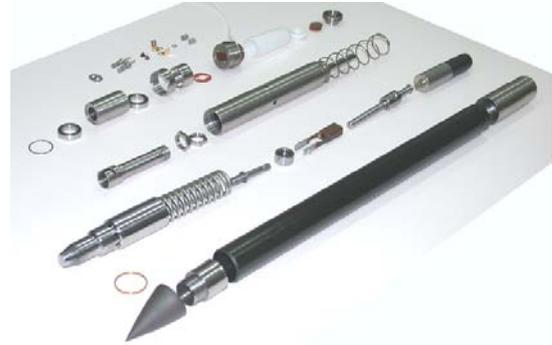
Figure 2 Mechanical parts of the mole KRET
