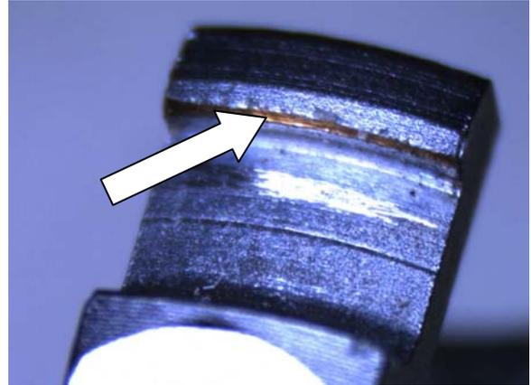
Fig. 4 Final abrasion effects on the latch working edge
