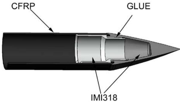
Figure 6 Joints of the CFRP tube with a metal tip
