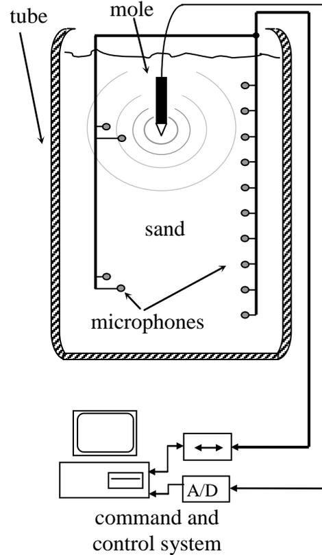
Figure 10 Mole testbed system: tube with dry quartz sand, distributed microphones and command and control system.
