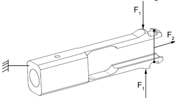
Fig. 3 The constrains and forces acting on the latch:
