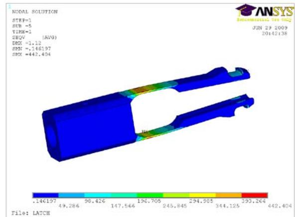
Fig. 5 Von Mises stresses in the latch
