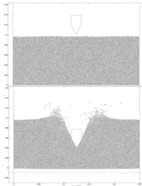
Figure 8 Snapshots of the penetrator motion for two different stages: before impact and during penetration.
