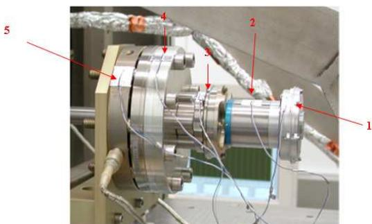
Figure 3.11: Thermocouple Measurement Positions
