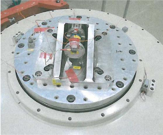
Figure 3.10: Arrangement of ECD on shaker table
