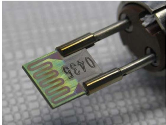
Figure 8 Thermal Knife after cutting tests
