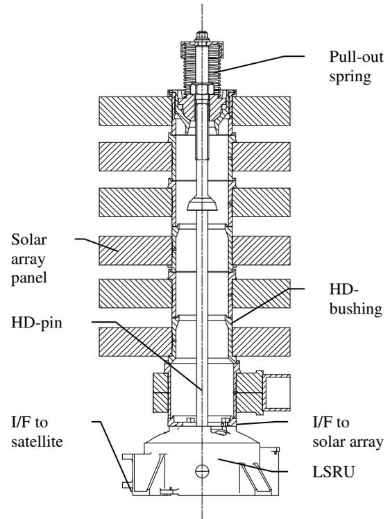
Figure 2-1: Cross-sectional view of integrated HD-stack (Alphasolar solar array design)
