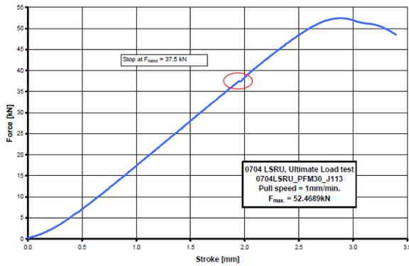
Figure 3-11: Force vs. stroke diagram (ultimate load test)
