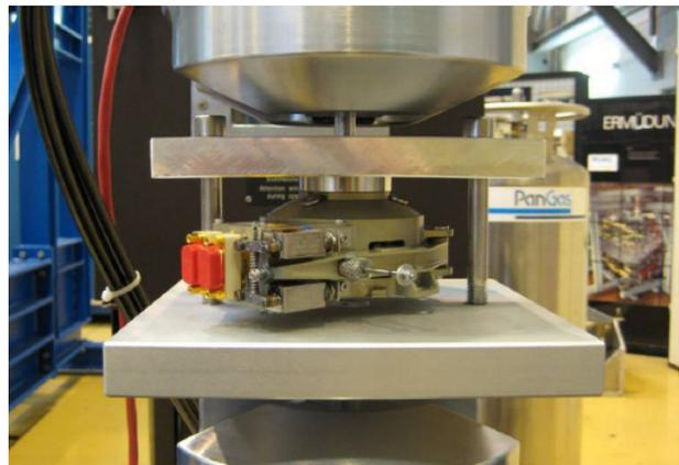
Figure 3-10: Setup for ultimate load test
