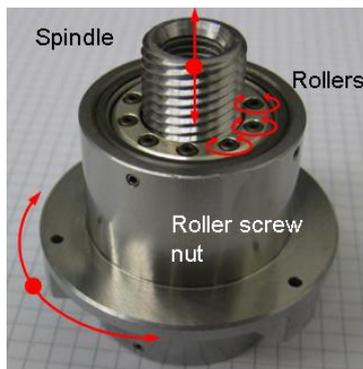
Figure 1-1: Roller screw assembly
