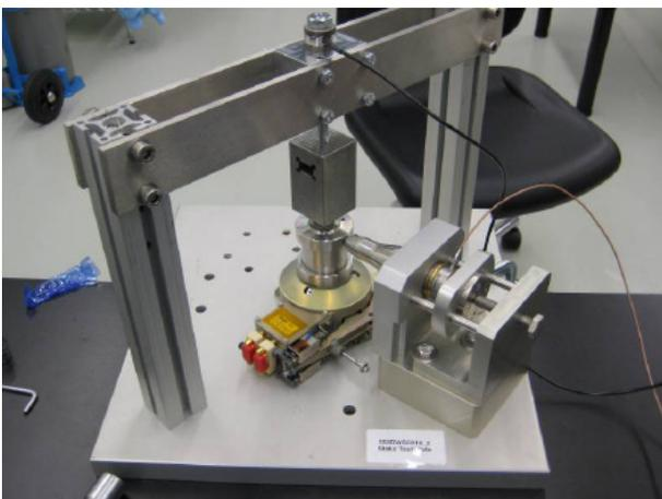
Figure 3-8: Setup for static test on housing (til rupture)
