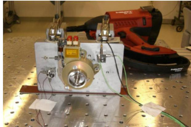
Figure 3-5: External shock test setup (in-plane)
