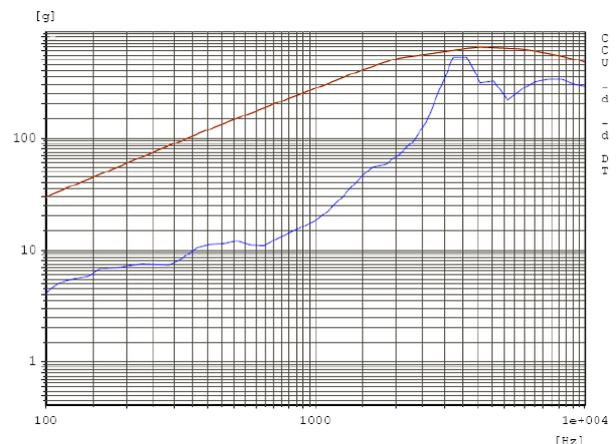
Figure 3-3: SRS, pos. 2x, 100 mm from source, 1st run
