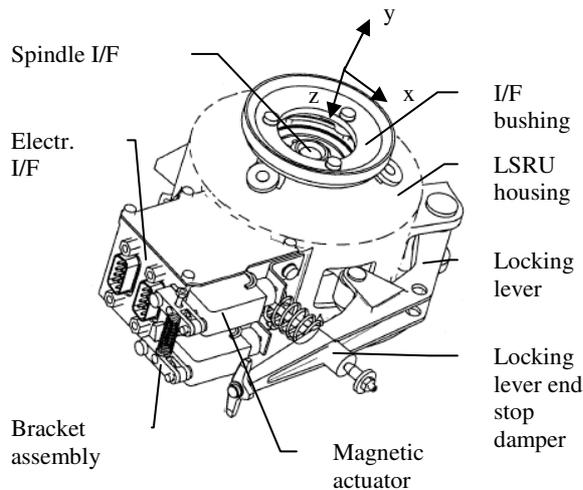
Figure 1-4: LSRU in unlocked condition
