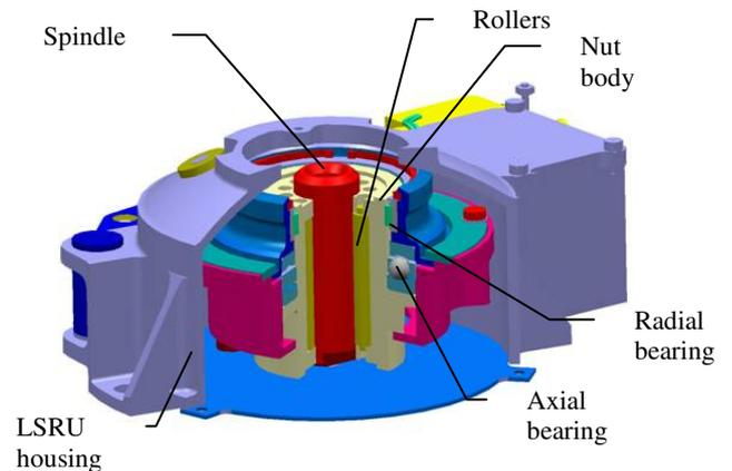
Figure 1-2: Cross-sectional view of LSRU
