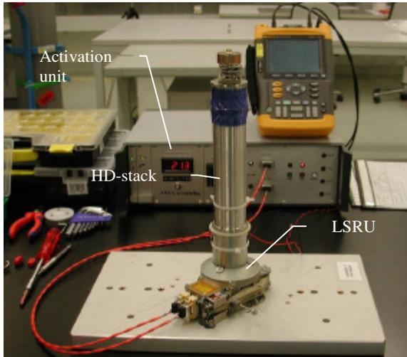
Figure 3-1: Setup for LSRU functional performance test
