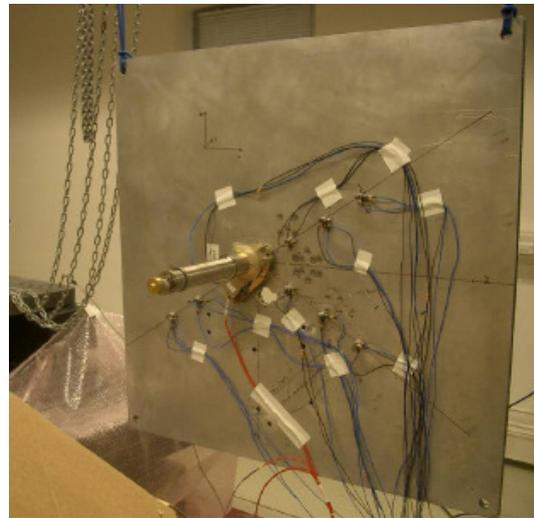
Figure 3-2: Test setup for output shock measurement
