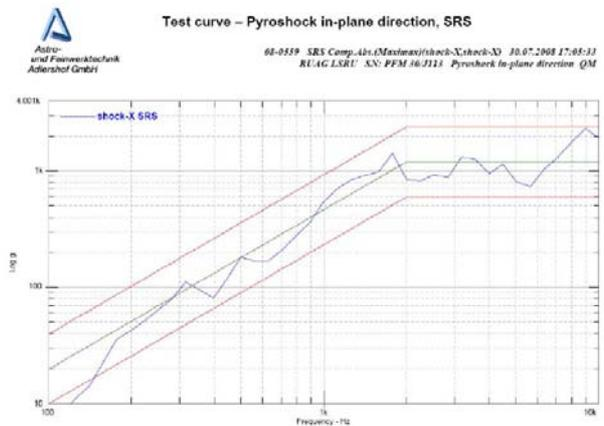
Figure 3-6: Shock level (SRS), in-plane excitation
