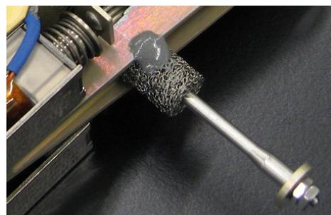
Figure 3-4: Locking lever end stop damper
