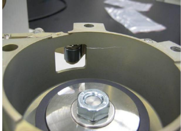
Figure 3-9: Broken LSRU housing (after static test 2)
