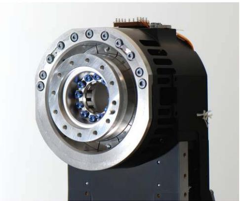
Figure 9. Bearing integrated into Wheel Support Mechanism.
