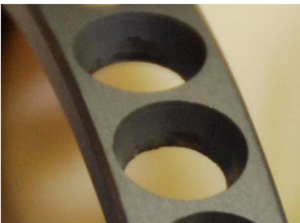
*Figure 3. Wear Marks inside the Cage Pockets.*
