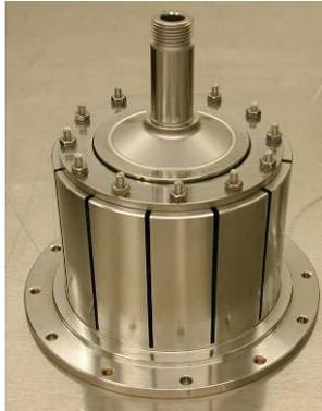
Figure 5. Isostatic Bearing Mount for Cryo Testing.
