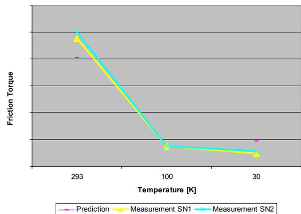
Figure 4. Measured Friction Torques.
