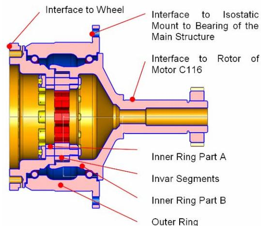
*Figure 1. Bearing Cross Section.*
