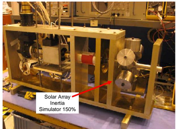
Figure 6 Inertia Testing Setup
