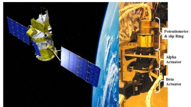
Figure 1 Glory Observatory and the Solar Array Drive Assembly
