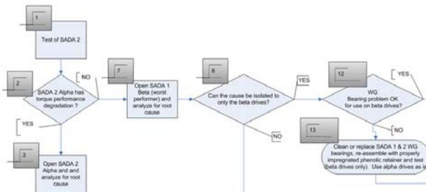
Figure 8 Initial Steps in a Detailed Test Strategy
