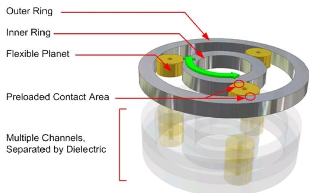
Figure 1: RCC Basic Geometry
