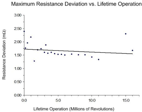
Figure 10: Operational Life Noise Performance Trend. Maximum resistance deviation was observed to trend downward with prolonged continuous operation. Note that the increase in resistance deviation at 15 million revolutions was due to an extended period of in-operation; allowing contaminants to form on the contact surface. Following a second run in period, resistance deviation returned to nominal levels.
