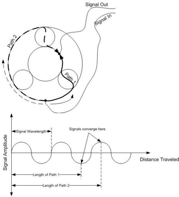
Figure 4a. Signal Path Length Difference (Top)
