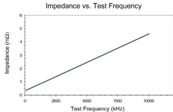
Figure 6: Three Planet RCC Series Impedance vs. Test Frequency. At 1 MHz, the series impedance was found to be less than 0.5  $\Omega$ , indicating the ability of RCC devices to transmit analog signals with higher frequency components.
