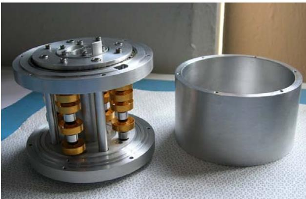
Figure 2. RCC Subassemblies (Dimensions: 4" height x 4.5" diameter)
