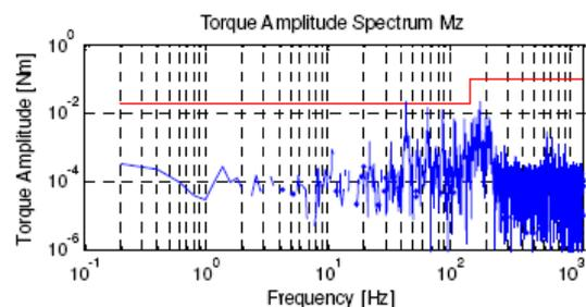
Fig. 22 Induced Torque Spectrum about Motor Rotation Axis
