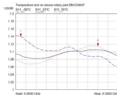
Fig. 10 RJ VSWR over Frequency
