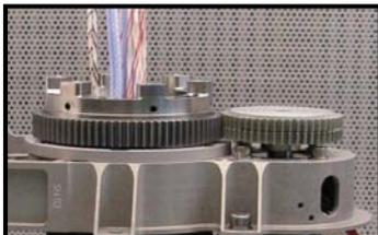
Fig. 7 Azimuth Gear Stage
