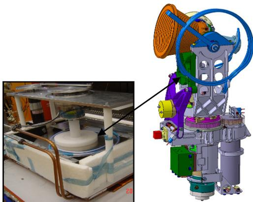
Fig. 3 Co-axial RF Harness, 540 deg Loop Life Test Configuration
