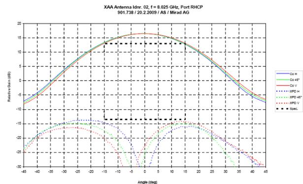
Fig. 15 Antenna Directivity Pattern 8.025 GHz
