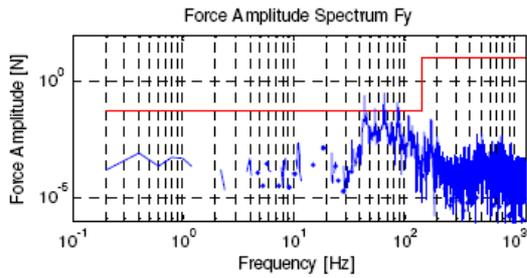
Fig. 23 Induced Lateral Force Spectrum
