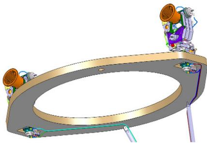
Fig. 1 Redundant APMs on S/C Platform
