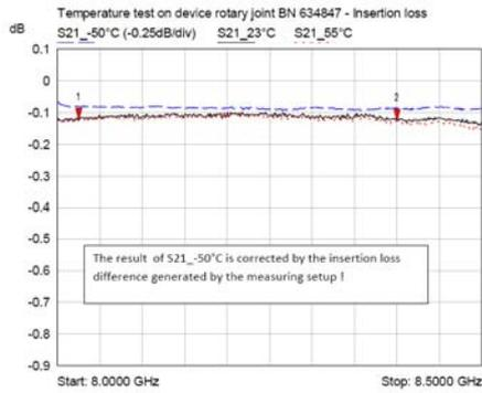
Fig. 11 Insertion Loss over Frequency
