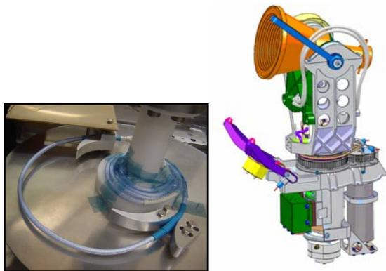
Fig. 2 Co-axial RF Harness Life Test Configuration 180 deg Loop
