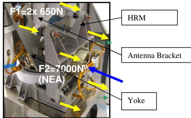
Fig. 17 Force Distribution on HRM H/W
