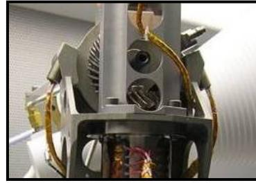
Fig. 8 Elevation Gear Stage
