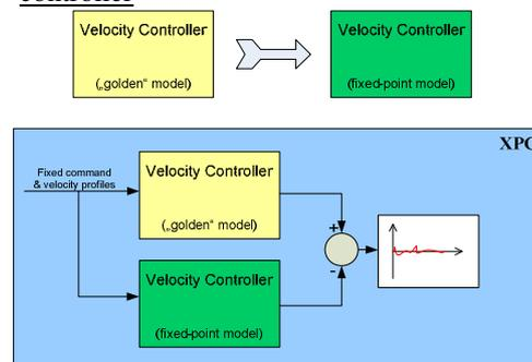
*Objective:* Generation of a velocity controller, fully basing on fixed-point arithmetic
