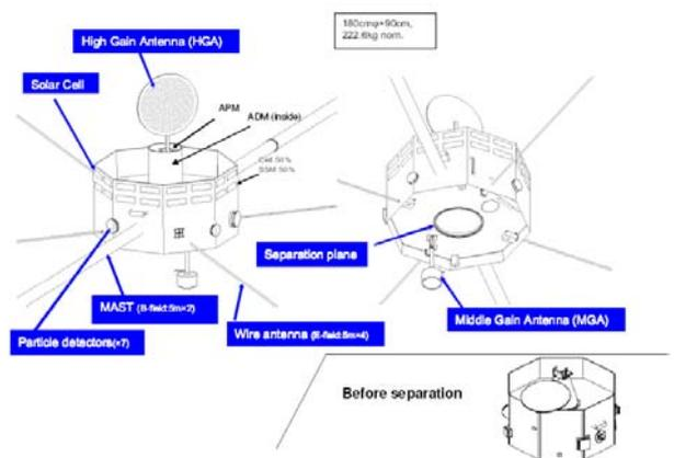
Fig.: 2 MMO S/C with HGA and ADM mounted on Top
