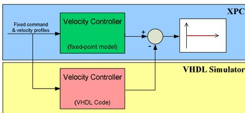
**Task:** Generation of VHDL code (FPGA source code) and Co-Simulation of fixed-point controller with VHDL behaviour
