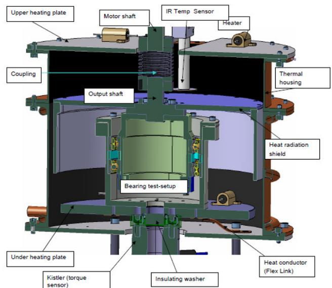
Fig.: 5 Flight Representative Bearing test stand and bearing configuration as used in the TV Test
