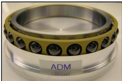
Fig.: 7 ADM Bearing, no degradation observed after Life test
