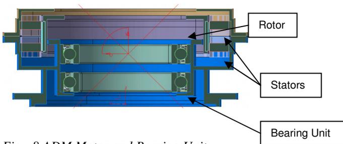
Fig.: 8 ADM Motor and Bearing Unit
