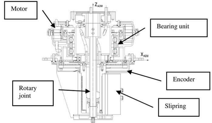
Fig.: 3 ADM Cross Section
