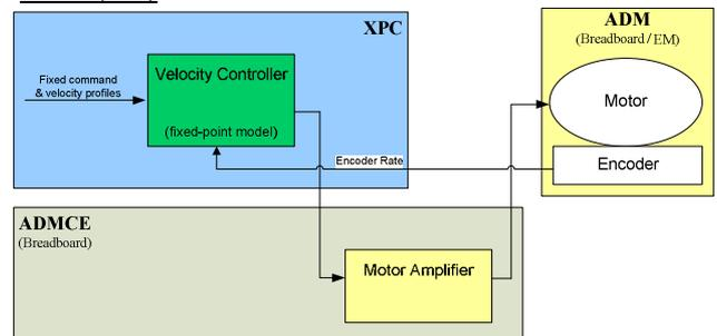
*Objective:* Full system verification of the ideal control performance. Simulation Model Verification and fine tuning
