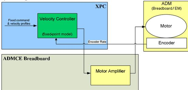
**Tasks:** Performance tests with fixed-point controller
