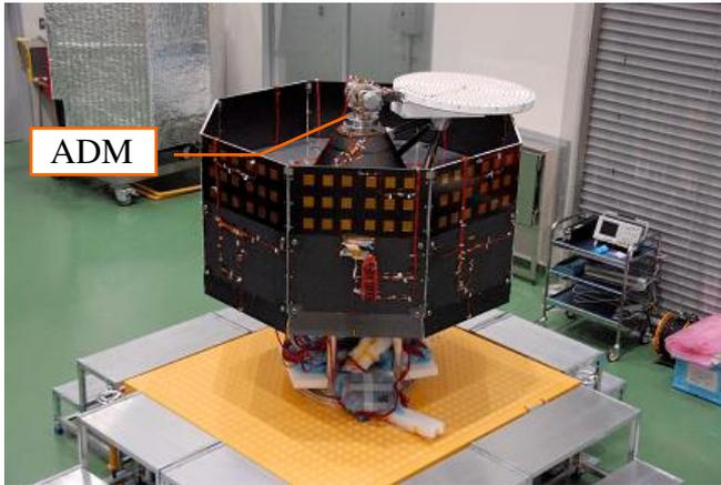
Fig. 3 MMO(MTM) and ADM mounting position
