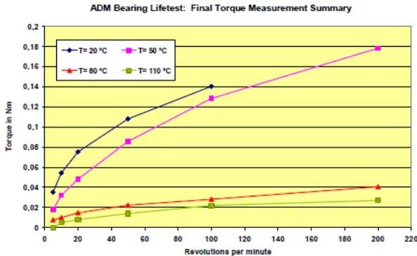
Fig.: 6 Friction Torque over rotation velocity at different temperatures (after 14 Million revs)
