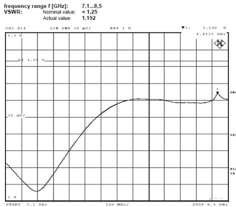
Fig.: 10 Rotary joint RF Performance at 110 deg C
