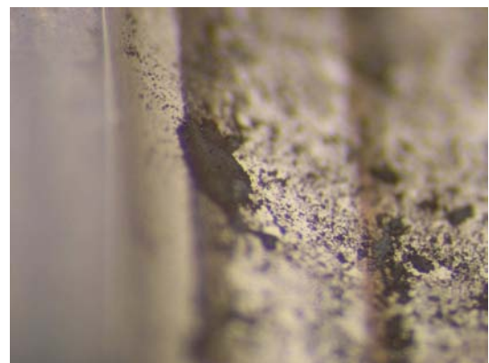
Figure 12 Wear particles on POLDER race
