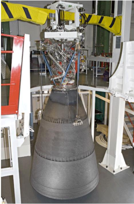
*Figure.18 shows the Vinci engine with the nozzle extension during dynamic characterization and deployment tests at Snecma*
