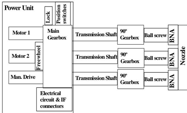
Figure 3 MDD block diagram
