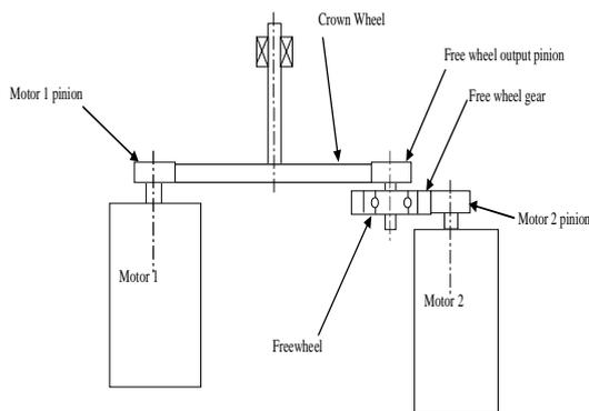
Figure 6 Motor1 and Motor 2 gearing arrangement
