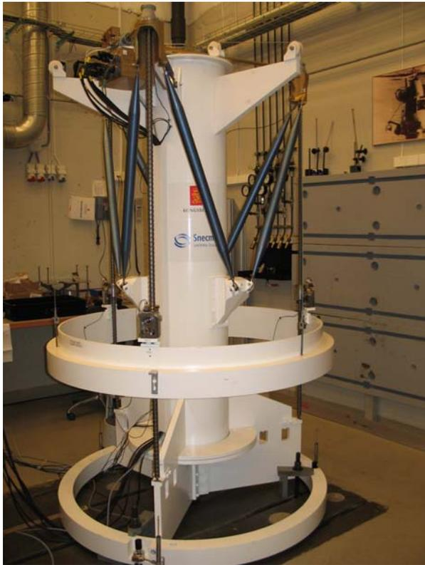
Figure 17. MDD-EM installed on the Test-Jig at KDA.
