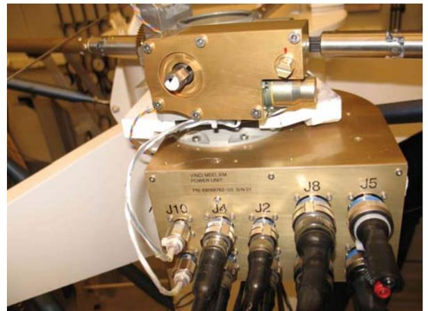
Figure 11. Locking Mechanism installed on the Power Unit
