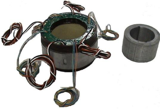
Figure 5. Quadruplex redundant BLDC torque motor
