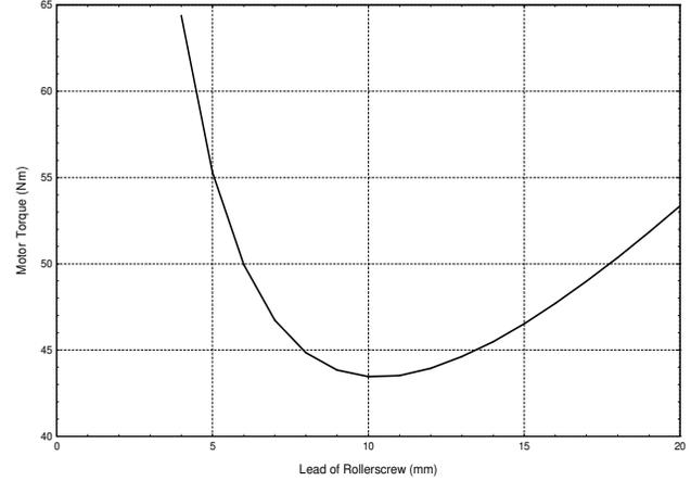
Figure 7. Optimum lead of Rollerscrew
