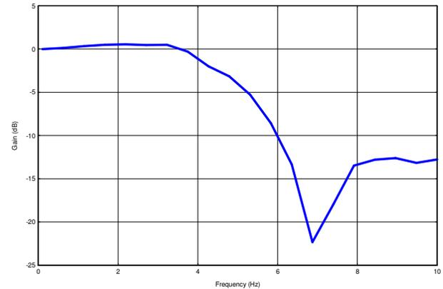
Figure 12. Frequency response of stage-2 EGC system
