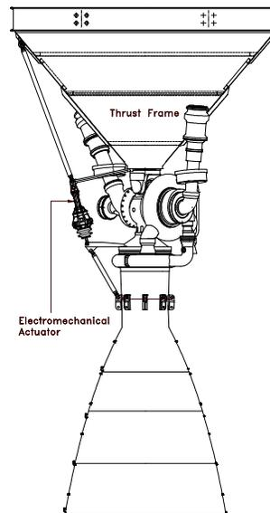
Figure 1. Stage-2 Engine Gimbal Control System
