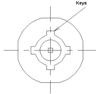
Figure 4. Rotary to linear conversion keys
