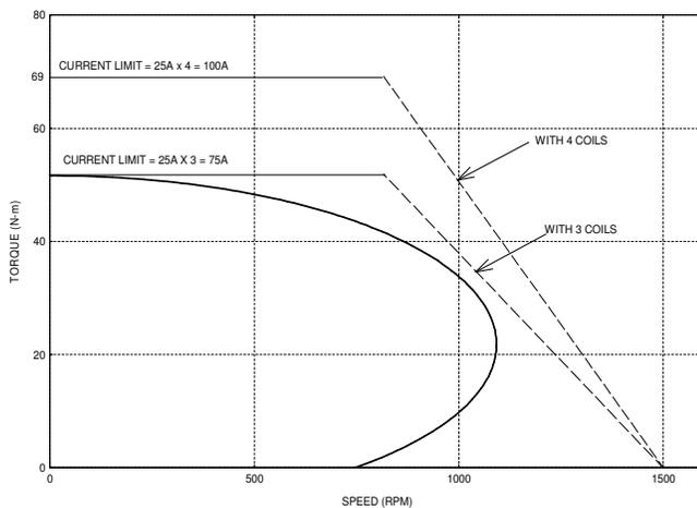
Figure 9. Load Locus of motor for STAGE-1 EGC system
