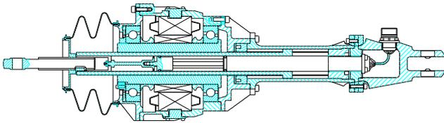
Figure 2. Stage-2 EGC Electromechanical Actuator
