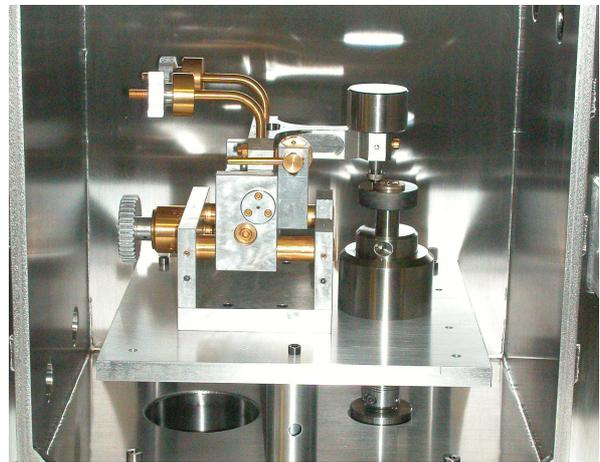
Figure 5. Vacuum pin-on-disc tribometer
