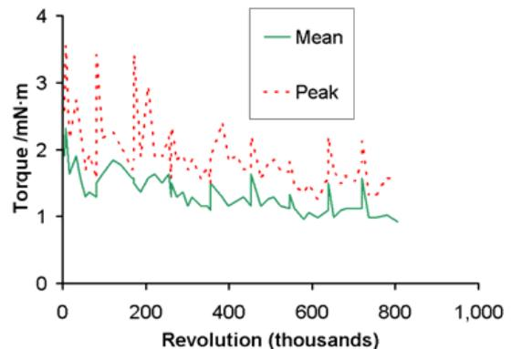
Figure 4. Lifetest results of bearing lubricated with  $\text{MoS}_2$  lubrication (balls & races) and titanium-Sintimid cages, running at  $275\text{deg.C}$  under vacuum [2]
