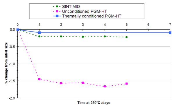
Figure 1. Dimensional change of dummy PGM-HT cages after heating to 250 °C – showing beneficial effects of pre-conditioning on PGM-HT. Sintimid 15M also shown on plot [2]
