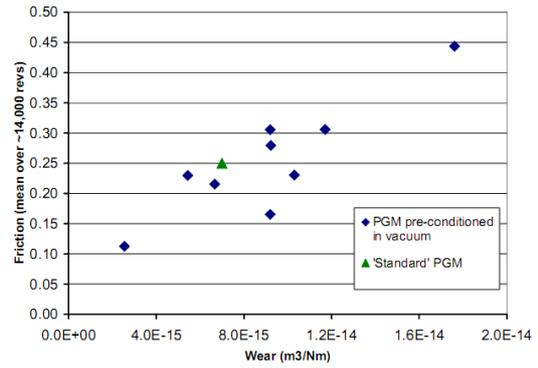
Figure 3. Integrated friction against wear rate. In-vacuum data from [5], 'Standard' data from [1]. Test performed under vacuum, load 5N, speed  $0.1\text{ms}^{-1}$
