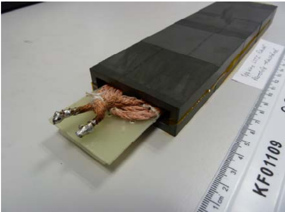
Figure 10. Prototype Transformer showing Litz Wire windings
