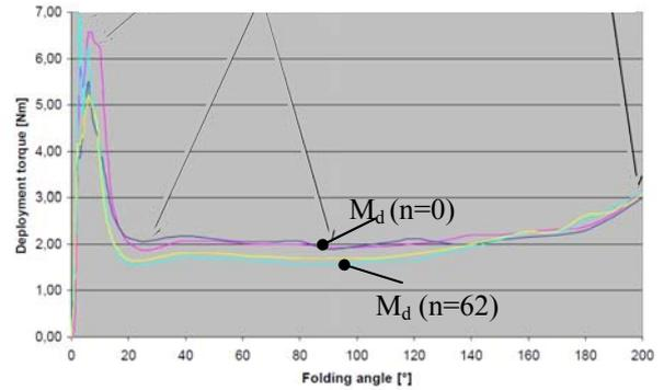
Figure 3. Deployment Torque Test Results.
