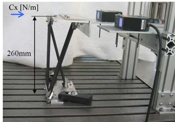
Figure 4. Stiffness Measurement Set-Up.
