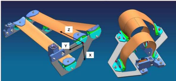
Figure 2. Unique Spring Blade Layout.
