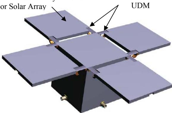
Figure 6. UDM used to deploy VHF Antennas (Could also be used to deploy Solar Arrays).
