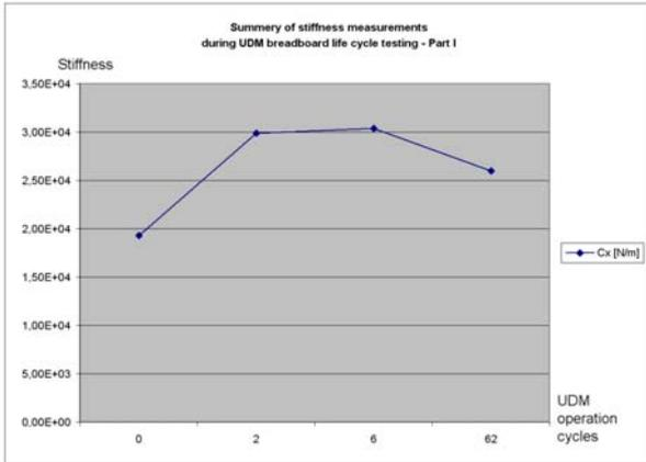
Figure 5. Stiffness Test Results (Cx [N/m]).
