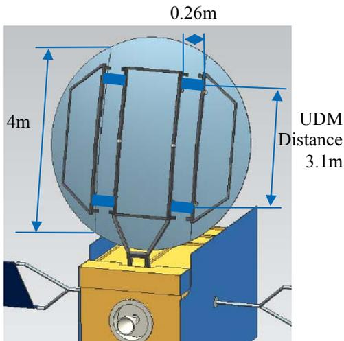
Figure 1. Proposed UDM Integration on Backing Structure of Reflector Antenna.
