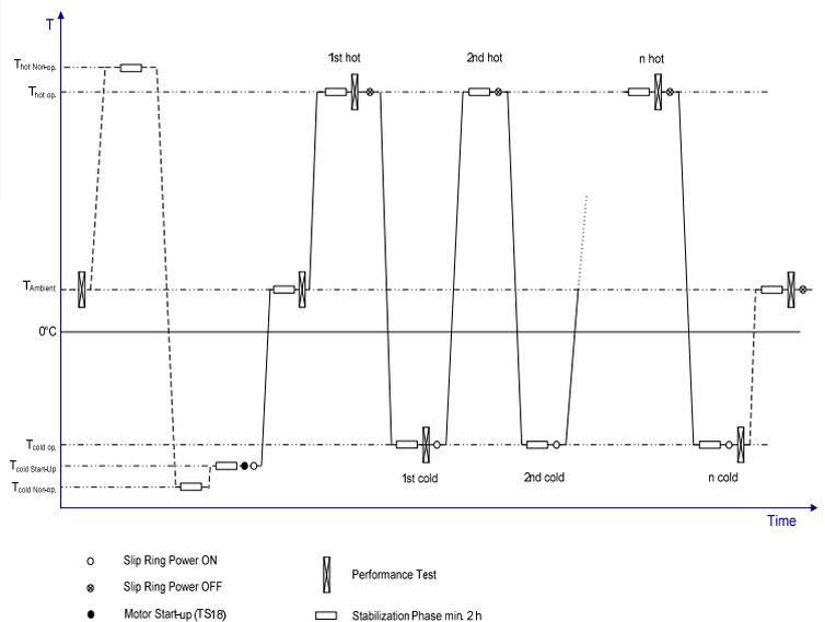
Figure 12: TV Cycling Tests
