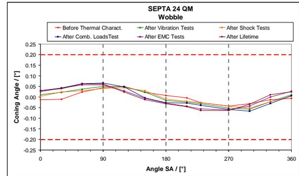
Figure 7: SADA Coning Error
