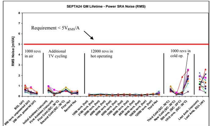
**Figure 13: Power SRA Noise (RMS Values) Evolution during Lifetime**
