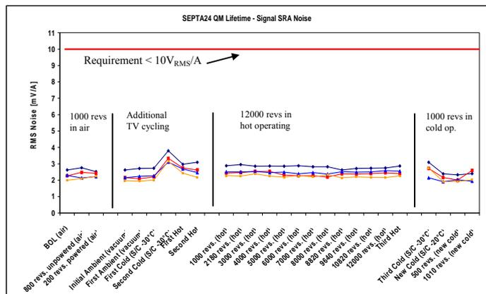
**Figure 14: Signal SRA Noise (RMS Values) Evolution during Lifetime**
