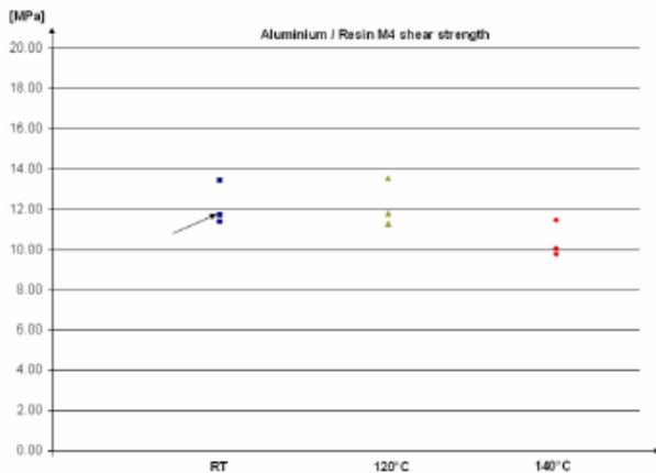
Figure 6: Aluminium on Rotor Resin Lap Shear Tests
