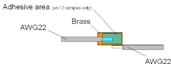
**Figure 4: Solder Joint Sample Configuration**
