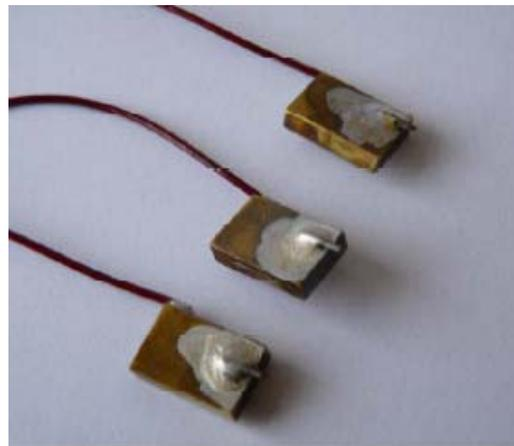
**Figure 5: Solder Joint Sample after Pull-Out Tests**
