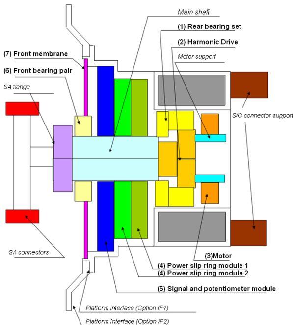
Figure 2: Configuration of the SEPTA<sup>®</sup>24 SADA
