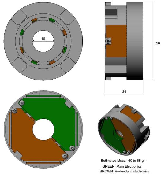
Figure 2 : the Stator (Top, Side, and Bottom views)
