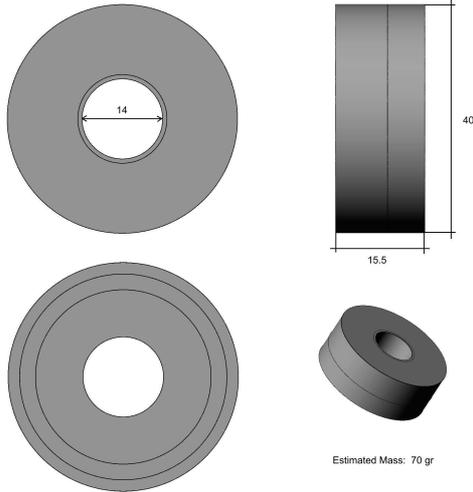
Figure 3 : the Rotor (Top, Side, and Bottom views)
