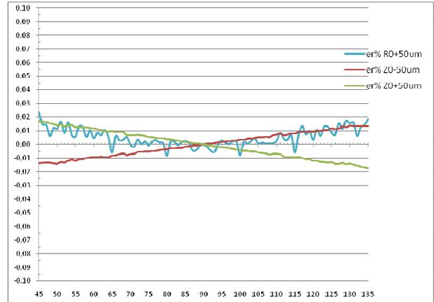
Figure 13 : er% as result of 50um axial and radial displacement
