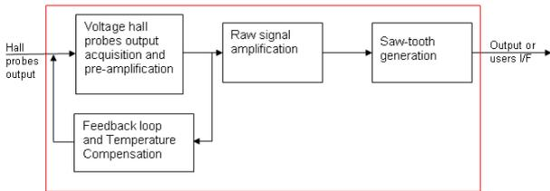
Figure 7 : Electronic design block diagram
