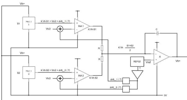
Figure 9 : Principle of operation of the Temperature compensation circuit
