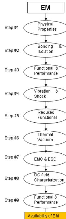
Figure 15 : Flow chart of the test sequence for EM INCAS step by step
