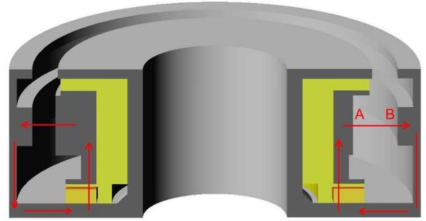
Figure 6 : perspective section view of the rotor's circular magnetic circuit
