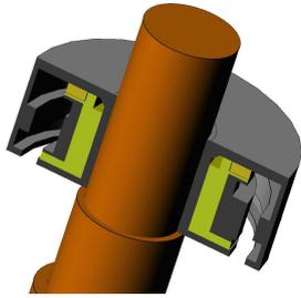
Figure 4 : the Rotor coupled to the Shaft
