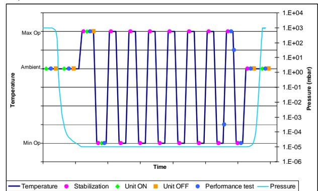
Figure 16 : Test profile for the thermal vacuum test
