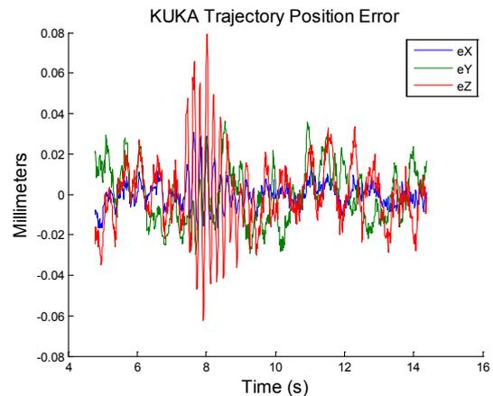
Figure 7. Sample test case of KUKA trajectory tracking while experiencing a force disturbance.
