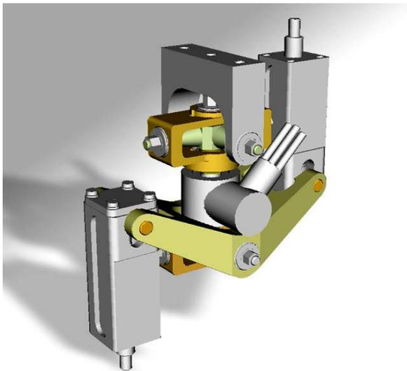
Figure 1. Load cell (with overload protection) assembly.
