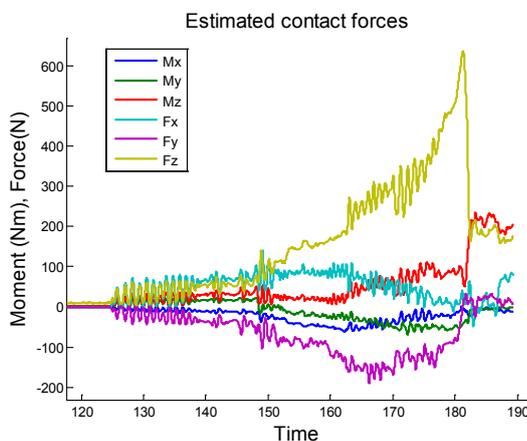
Figure 9. Contact force wrench from test trajectory 5.
