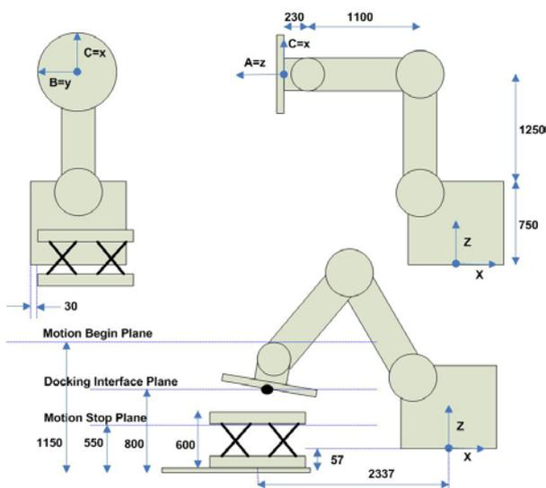
Figure 4. KUKA and IBDM coordinate frames and motion planes schematic.
