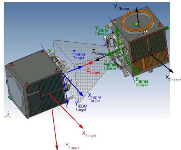
Figure 3. Lightweight Vehicle Docking.
