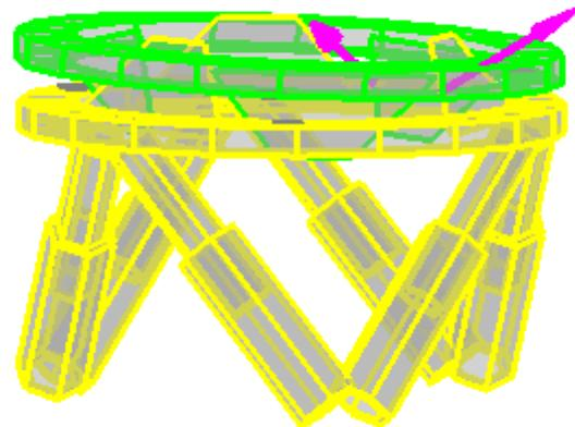
Figure 4. Passive (green) and active (yellow) IBDM simulation animation model with interacting contact forces (purple).
