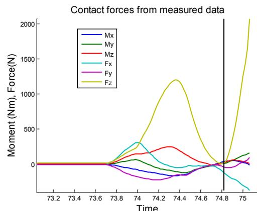
Figure 11. Measured load cell forces from test trajectory 5.
