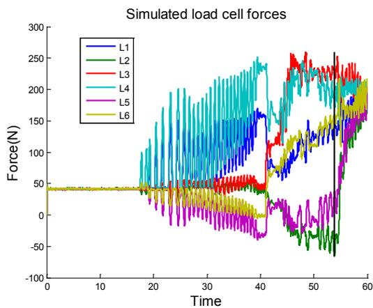
Figure 5. Simulated load cell forces during contact for Test Case 5.
