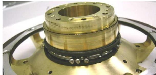
Figure 12. QM1 upper bearing cage post life test
