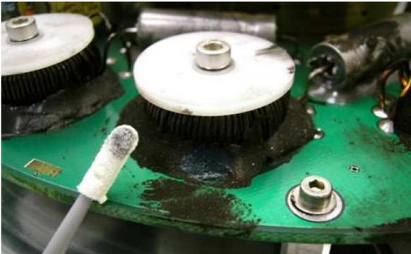
Figure 13. QM1 debris over wheel electronics
