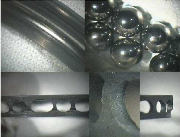
Figure 9. LTM upper bearing race, balls, cage post test
