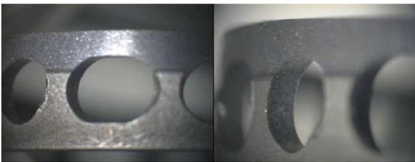
Figure 14. QM1 lower cage post life test
