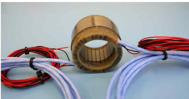
Figure 7: Sentinel-3 Scan Drive Motor stator with independent integral windings
