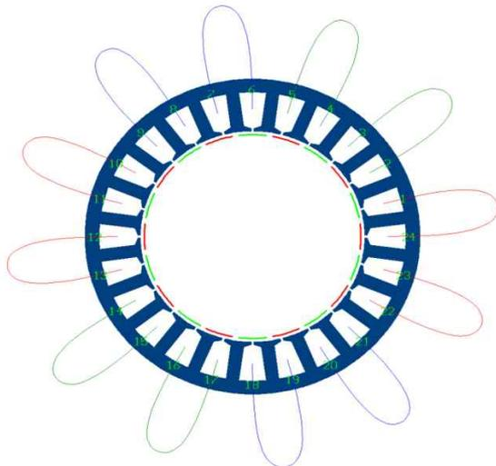
Figure 2: Physical separation of windings by winding every coil on a single tooth
