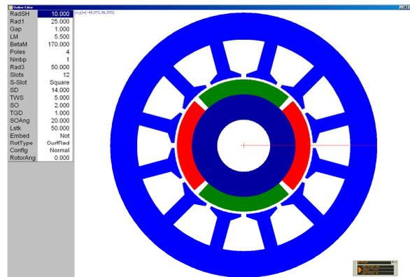
Figure 1: Analytical Design of a Brushless Motor using SPEED
