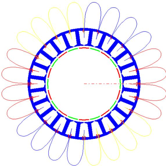
Figure 6: Winding scheme of Sentinel-3 Scan Drive Motor with 20 poles and 24 slots
