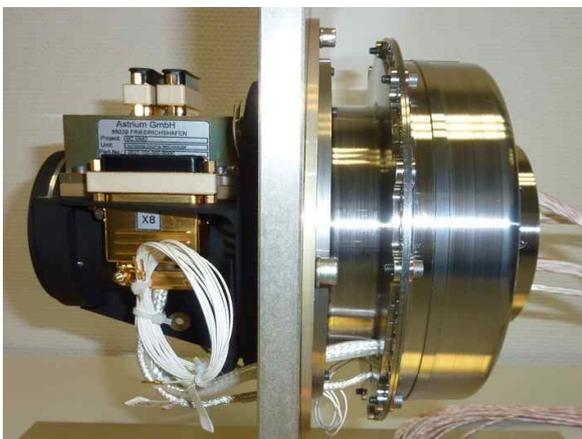
Figure 4: MMO Antenna Despin Mechanism
