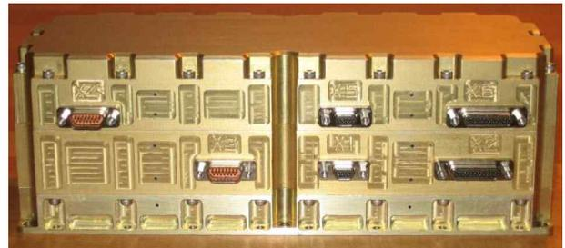
Figure 8: A 2-channel, single-level redundant Motor Control and Drive Unit with both dual motor, encoder and command channels
