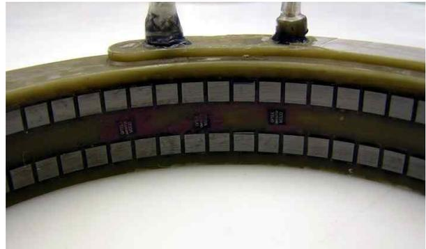
Figure 5: Main and redundant stator, potted as one unit
