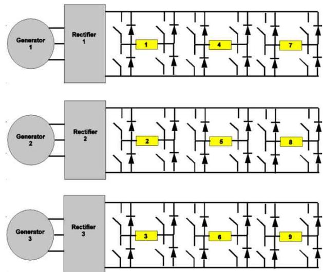
Figure 3: Full electrical isolation for a 9 phase drive with 2-level power supply redundancy
