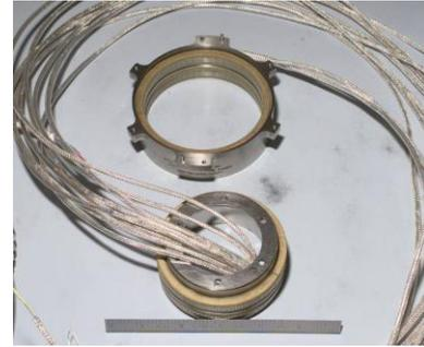
Figure 9. BAPTA 2-speed Resolver (1x/64x).
