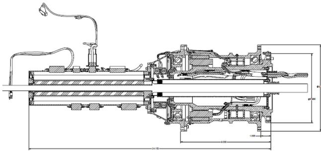
Figure 2. SMA Cross-section View.
