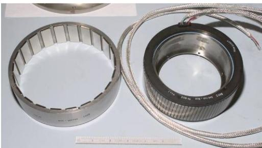
Figure 8. BAPTA (not GMI) 3-Phase DC torque motor.
