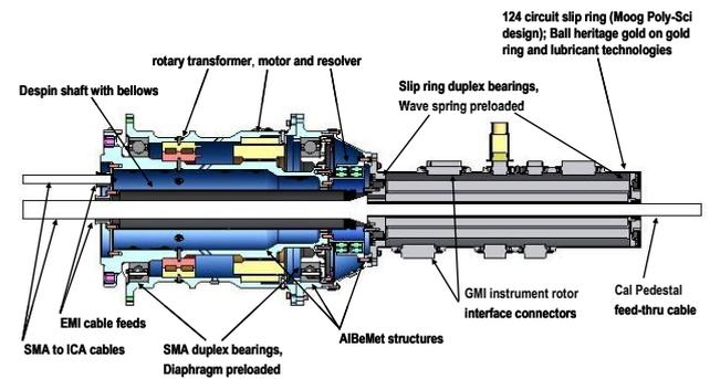
Figure 6. Cross-section of the SMA design with drive component labels.
