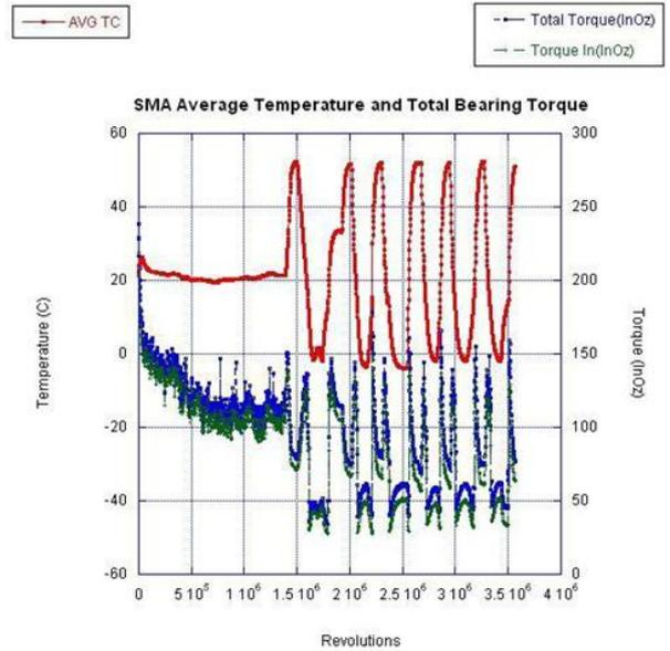
Figure 14. SMA main bearings life test temperature, bearing torque baseline over temperature, and total number of revolutions completed.
