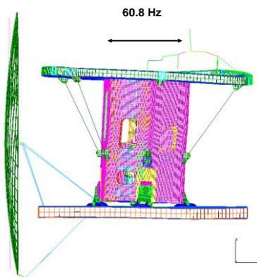
Figure 4. Finite Element (FEM) model of GMI instrument with SMA and launch restraints meets the first mode stowed frequency requirement (>50 Hz).
