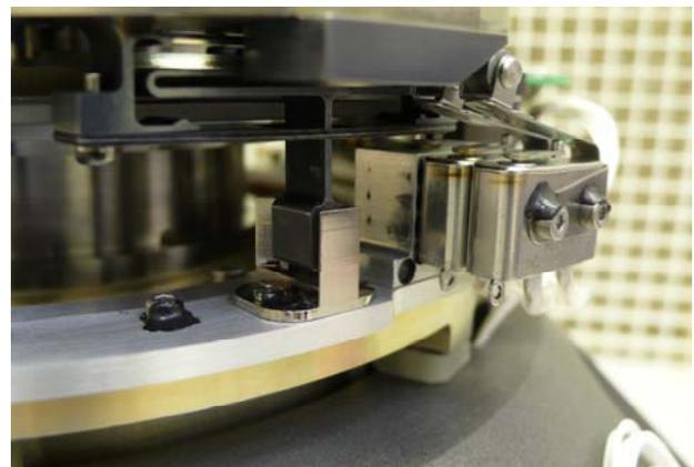
Figure 4. Flexible Magnet Arm in Detent Position
