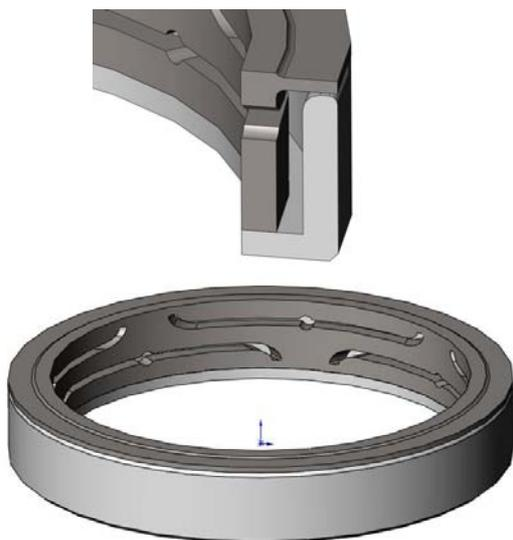
Figure 5. CTM Spring and Snubber Arrangement
