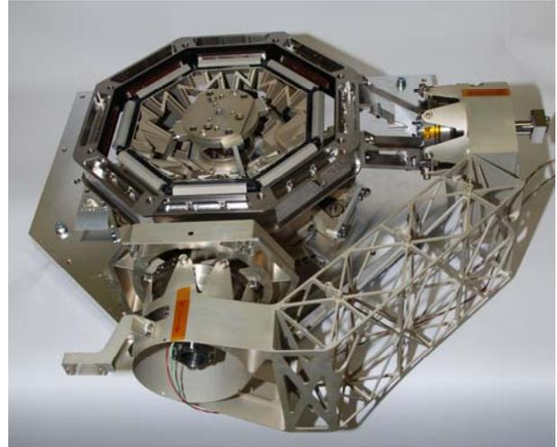
Figure 4. Pointing Arm attached to the HDRM
