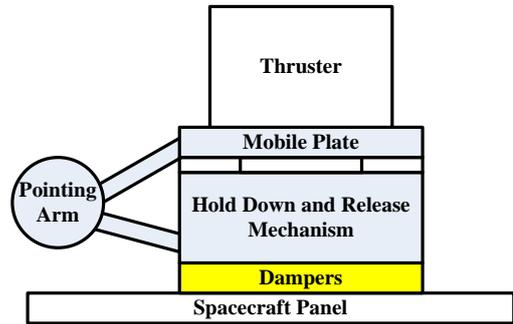
In this configuration the dampers are also directly in the load path of the stowed configuration, but also in the load path in the deployed configuration, making this design sensitive to aging of the damper material which then has to be carefully assessed. Aging of the damper material can be an issue if elastomere dampers are used.
