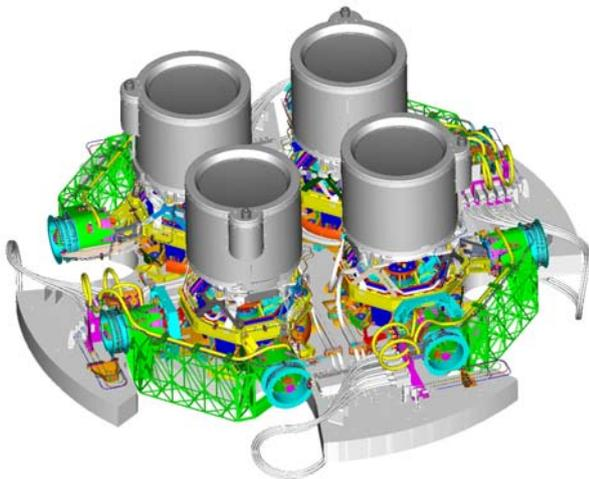
Figure 1. TPMs with Thrusters and Thruster Floor.
