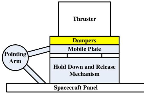
In this configuration the dampers are directly in the load path both of the stowed and of the deployed configuration. The dampers are close to the thruster. So the dampers are exposed to high temperature during operation. The long term stability of the dampers under such a thermal load may be an issue.
