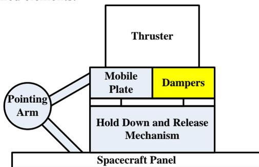
This configuration was used in the RUAG Thruster Pointing Mechanisms for Artemis (Ref. 1-3) and in the RUAG Thruster Pointing Mechanism for Eurostar 3000 (Ref. 4). The advantages of this configuration are that
