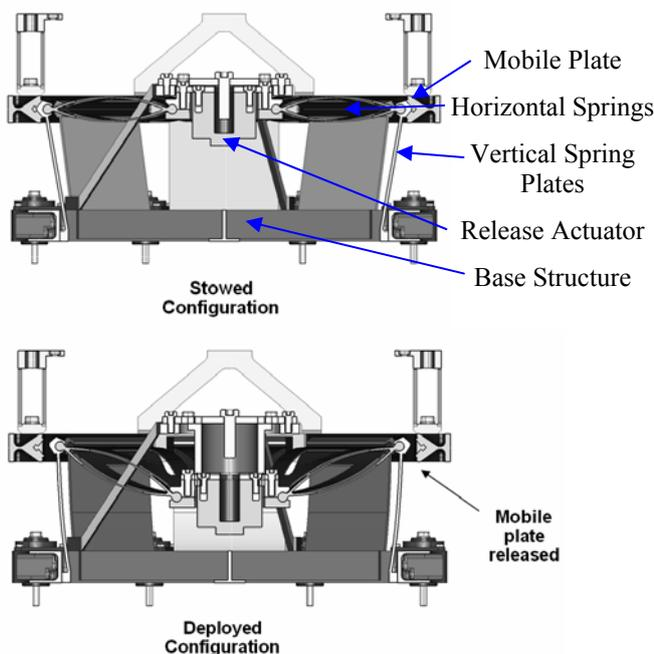
Figure 5. HDRM in stowed and deployed configuration (Principle Drawing)
