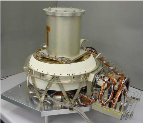
*Figure 6. Thruster Pointing Mechanism (TPM) with Thruster Mass Dummy and Sun-Shield attached.*
