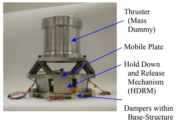
Figure 2. TPM Structure (Breadboard Model)
