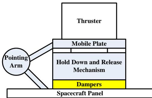
In this configuration the dampers are directly in the load path of the stowed configuration, but off the load path in the deployed configuration, again making this design insensitive to aging of the damper material.
