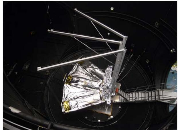
Fig. 13 QM DSA Deployed in LSS Solar Simulation
