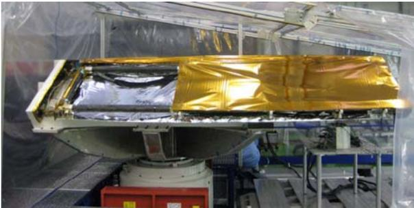
Fig. 10 QM DSA Z Axis Vibration Configuration
