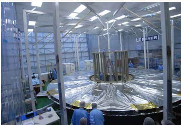
Fig. 1 Gaia Sunshield Deployed
