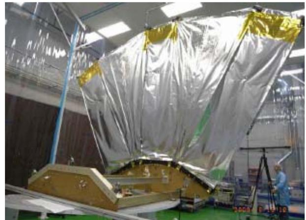
Fig. 9 QM DSA Horizontal Deployment Test
