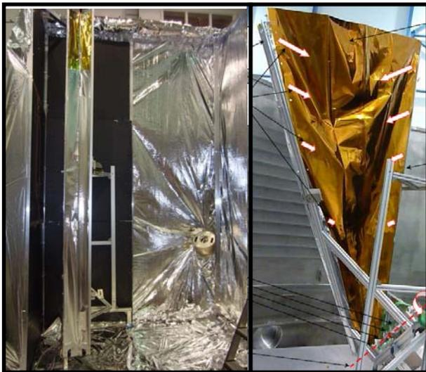
Fig. 14 Unrolling Test in VC (Stow & Deployed)
