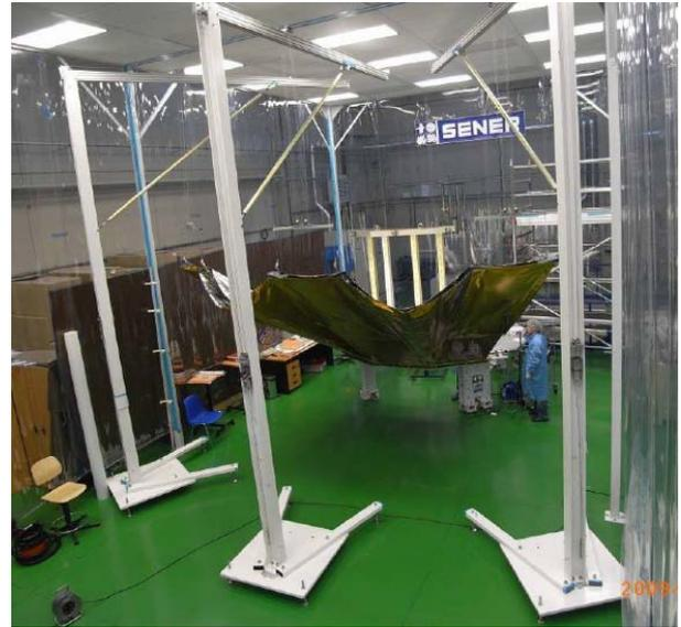
Fig. 8 QM DSA Vertical Deployment Test
