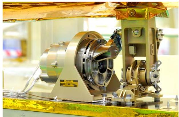
Fig. 15 DSA Actuator and Four-Bar-Linkage
