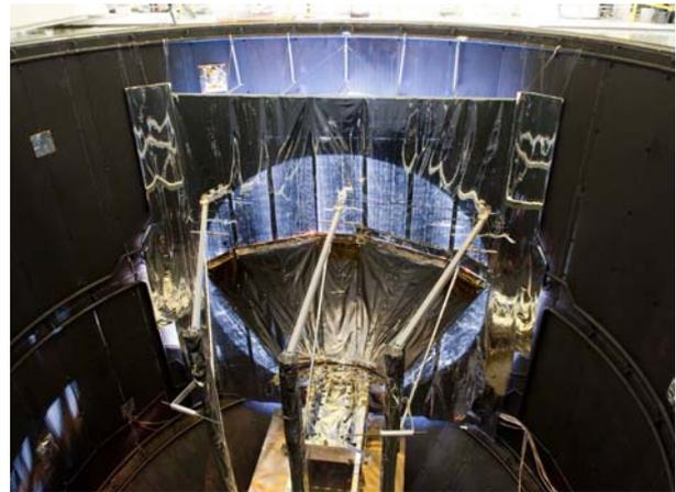
Fig. 11 QM DSA in LSS Solar Simulation
