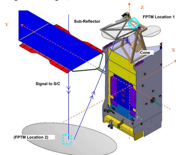
Figure 1. Cassegrain Configuration with Main ( $D=5m$ ) and Sub Reflector ( $D=2m$ ).
