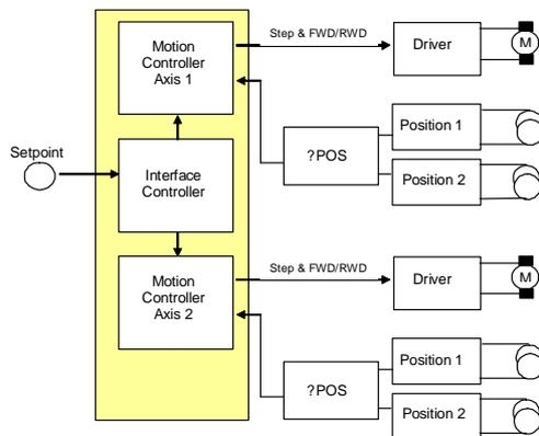
Figure 5. FPTM Drive Electronics Concept.
