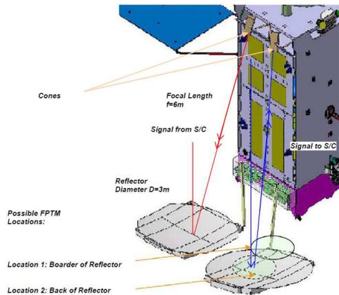
Figure 2. Single Offset Configuration with Main Reflector ( $D=5m$ ).
