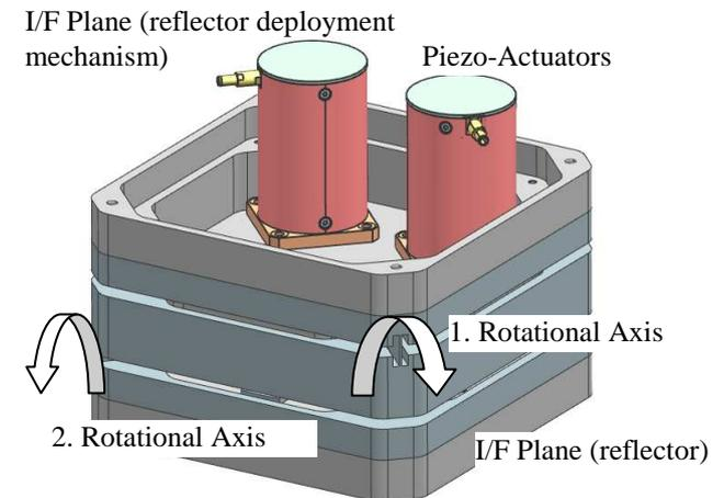
Figure 3. FPTM Monolithic Design Concept.
