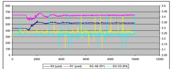
Figure 17: Thermal stability for large excursion in closed loop – 24°C → 40°C
