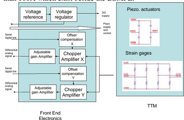
Figure 11: Front End Electronic Architecture
