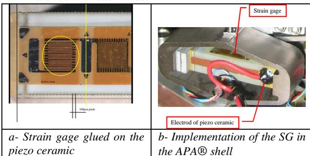
Figure 10: Integration of the strain gage onto the APA®
