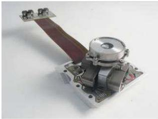
Figure 15: Realisation of the Tip-Tilt mechanism BBM
