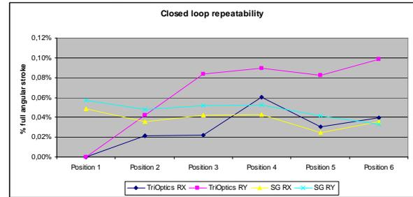
Figure 16: Repeatability results for any identical angle in closed loop
