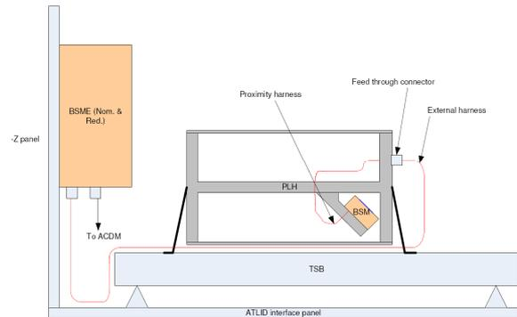
Figure 2 : BSA implantation schema
