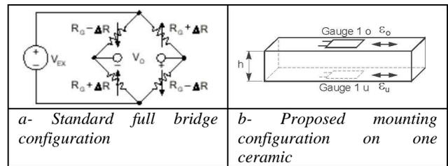
Figure 9: Selected Full bridge configuration and its application on the push pull piezomechanism
