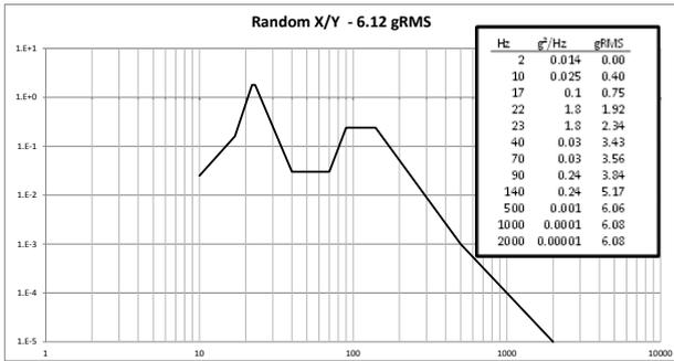
Figure 23 – X,Y Random levels [ $g^2/Hz$ ]
