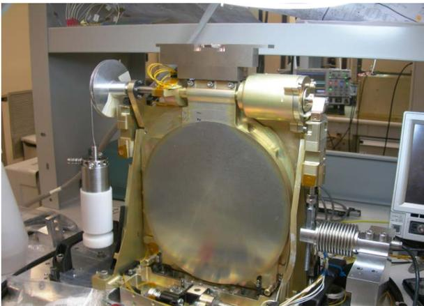
Figure 19 - Force measure setup for EAD opening
