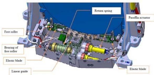
*Figure 11 – Launch Lock Device - Locking position*
