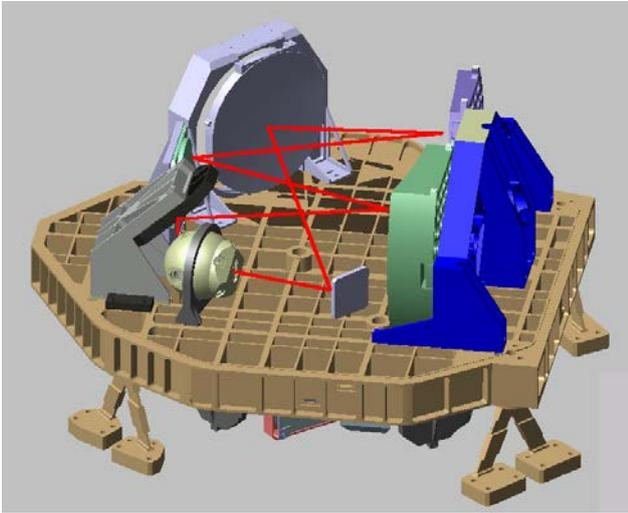
Figure 2 – PRISMA spectral calibration optical path
