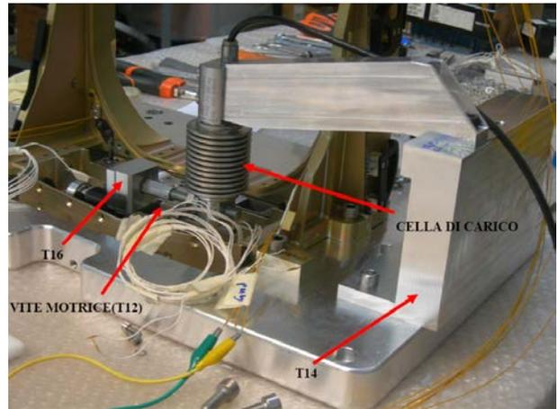
Figure 20 - Force measure setup for LLD
