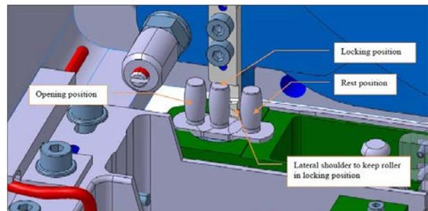
*Figure 13 – different pin engagement position*
