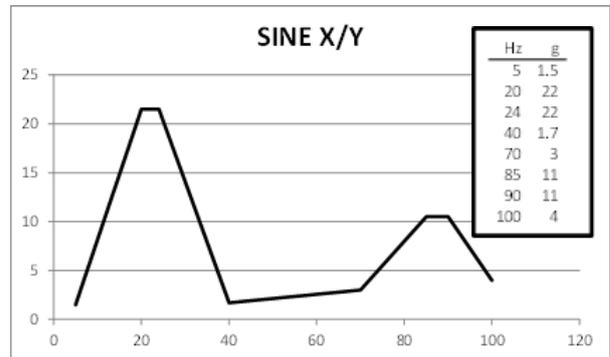
Figure 21 – X,Y Sine levels [g/Hz]
