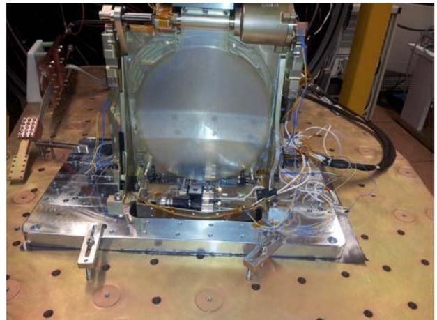
Figure 27 – MPM mechanism inside Thermal vacuum chamber
