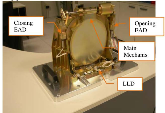
*Figure 16 - Main Port Mechanism (inside view)*
