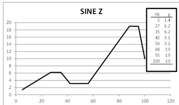
Figure 22 – Z sine levels [g/Hz]
