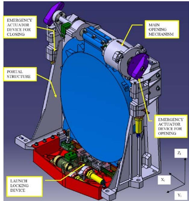
Figure 3 – MPM in closed position
