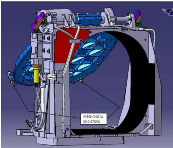
Figure 8 – Mechanical end stops for Port positioning
