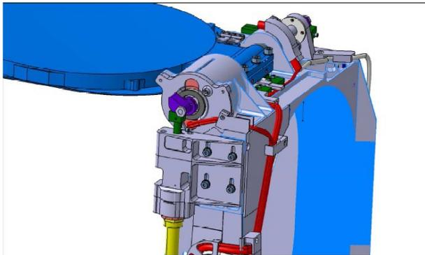
*Figure 15 – emergency opening system - Port in open position*
