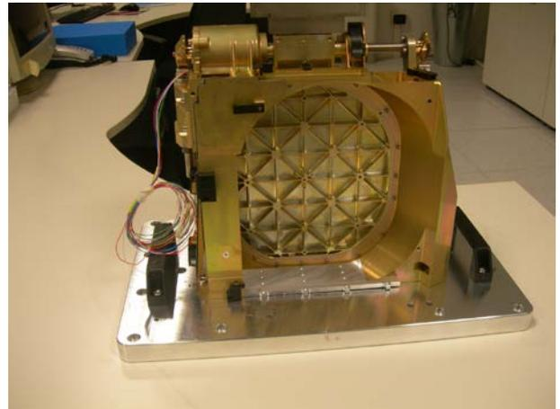
*Figure 17 - Main Port Mechanism (outside view)*
