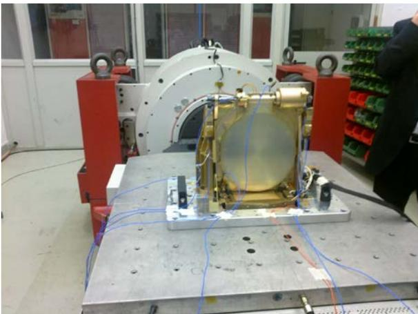
Figure 25 - Mechanical Vibration X,Y-axes
