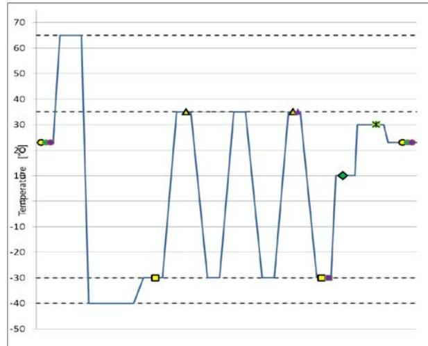
Figure 26 – Thermal vacuum cycling
