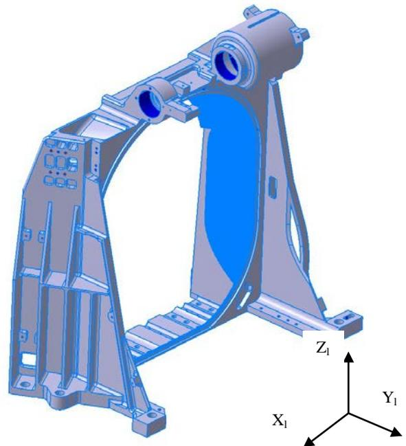
Figure 6 – Aluminum Portal Structure
