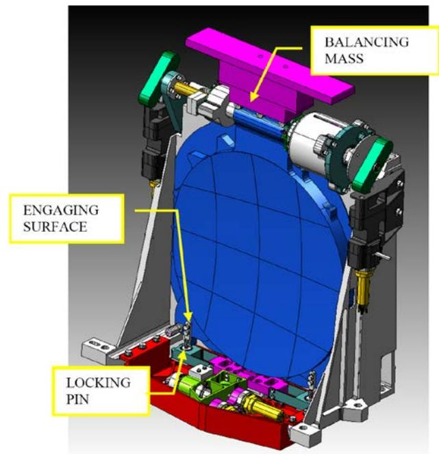
Figure 10 – Cover balancing mass
