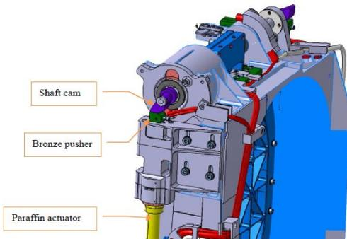
*Figure 14 – emergency opening system - Port in close position*
