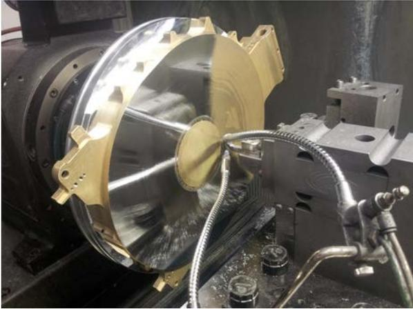
Figure 7 – Port optical diffuser machining
